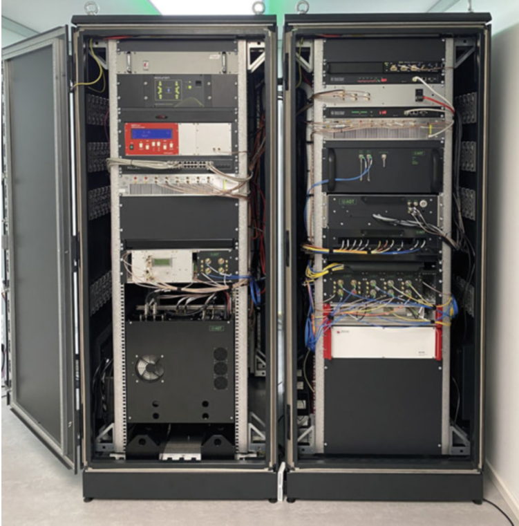
Fig. 8 A photograph of the MARMOT system which is a 19"-rack-mounted room-temperature quantum computer, having a less than 2 m 2 footprint and a power consumption of less than 2 kW. Designed for the installation at HPC infrastructures and data centers, the PINE setup is located behind a front plate on the bottom of the left rack, while the full laser system and stabilization is placed in the right rack
