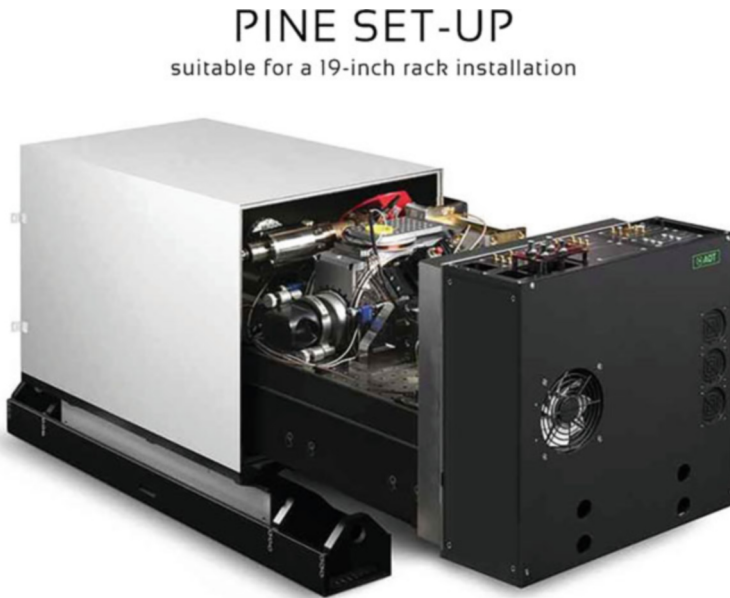
Fig. 7 This configuration of the PINE setup is ready to be mounted into a standard 19" rack with easy access by mounting it on sliding rails which act as a drawer that can be pulled out of the rack. Additionally, it features a vibration isolation stage, a scientific camera for imaging purposes, and an electromagnetic shielding structure
