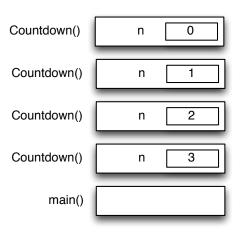
There is one instance of main() and four instances of Countdown(), each with a different value for the parameter n. The bottom of the stack, Countdown()
