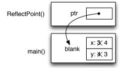
The parameter **ptr** is a reference to the structure named **blank**. The usual representation for a reference is a dot with an arrow that points to whatever the reference refers to.
