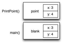
If PrintPoint() happened to change one of the member variables of point, it would have no effect on blank. Of course, there is no reason for PrintPoint() to modify its parameter, so this isolation between the two functions is appropriate.
