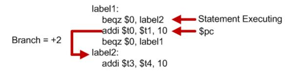
The second branch instruction branches backward to label1. In this case, the distance between the instruction and the label is -2 instructions, which is 2 words or 8 bytes, back from the current
