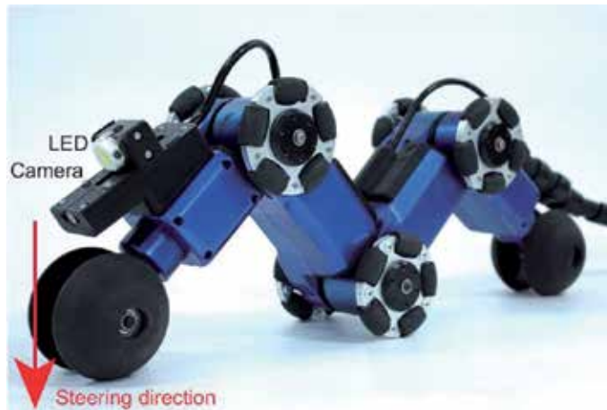
Figure 12. AIrO-2.2 with a shadow-based operation assistant system [26].
