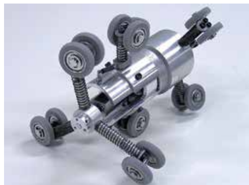
Figure 2. Screw-drive in-pipe mobile robot for 5-in pipelines [12].
