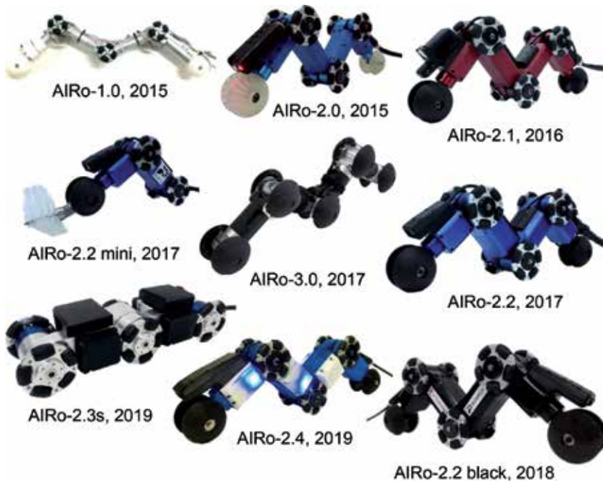
Figure 11. Multi-link-articulated wheeled-type in-pipe robots in the AIRo-series developed by the authors.
