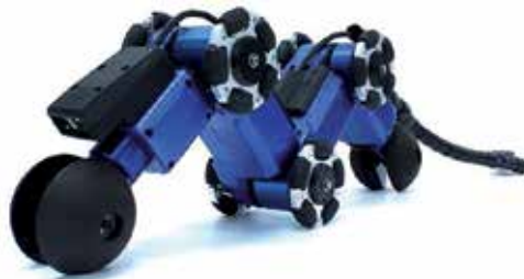
Figure 7. A multi-link-articulated wheeled-type in-pipe robot named AIRo-2.2 [20].
