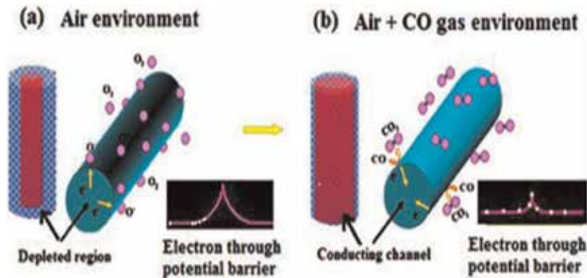
Figure 2. Schematic illustration of toxic chemical sensing process. (a) Adsorption of oxygen at surface of nanowires in air and creation of potential barrier and depletion region. (b) Modulation of potential barrier and depletion region after reaction of carbon monoxide (CO) at surface of n-type semiconductor.
