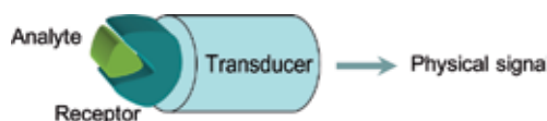
Figure 3. Illustration of a chemical sensor. (modified and adapted with permission from Ref. [103]. Copyright 2008, MDPI).
