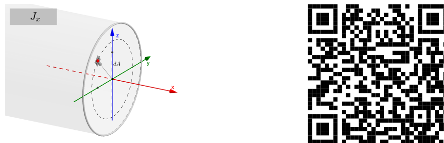
Figure 10.1.7 In-plane and out-of-plane rotation of element dA about the x , y and z axes.
