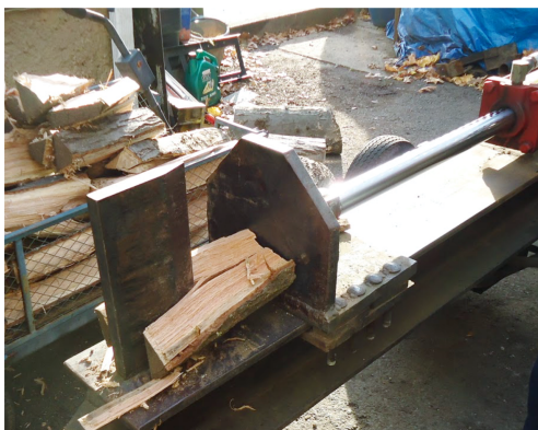
(a) A low friction wedge is used to split logs.
