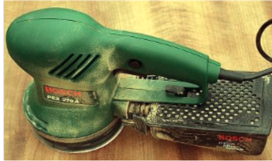
Figure 9.7.1 This orbital sander rotates a circular sanding disc against a stationary surface. The disc friction between the sanding disc and the surface exert a moment on both the surface and the sander.
