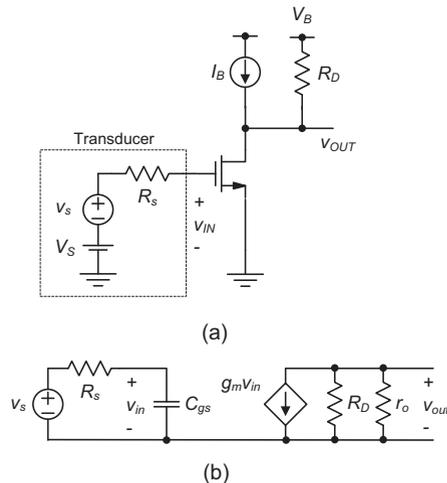
**Figure 3-7:** (a) Common-source amplifier driven by a transducer with finite source resistance. (b) Small-signal model with the intrinsic gate capacitance.
