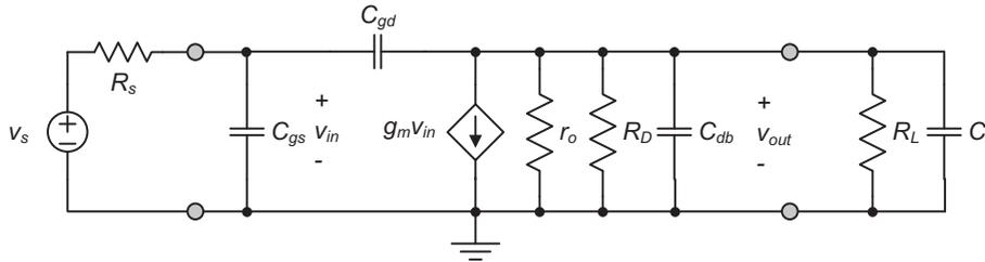
**Figure 3-22:** General two-port model for the common-source voltage amplifier valid at high frequencies.
