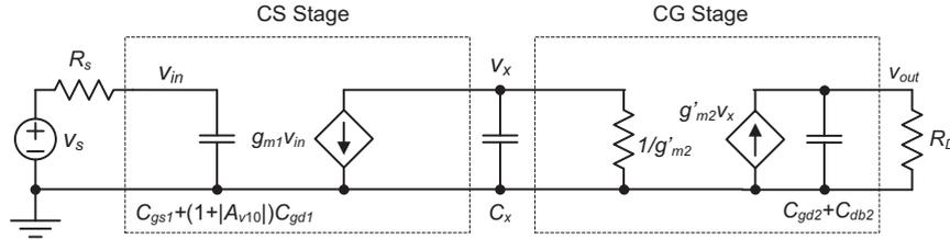
**Figure 6-10:** Unilateral model of the cascode amplifier.
