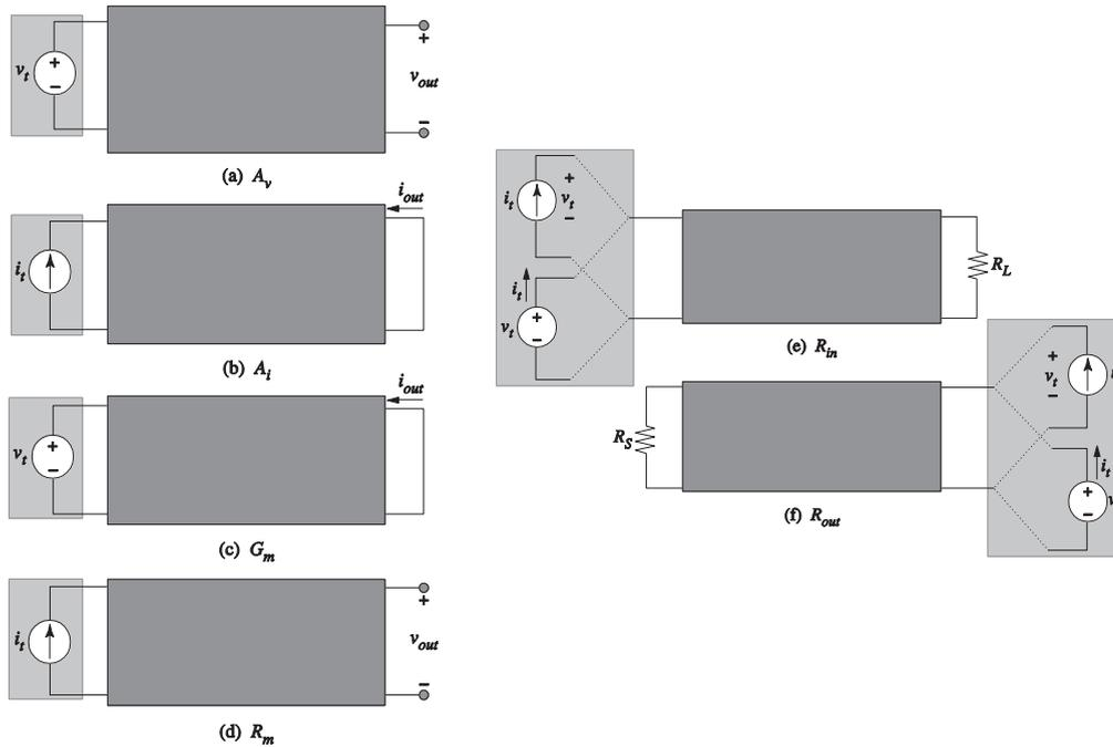
**Figure 1-13:** Method to calculate two-port amplifier model parameters: (a) voltage gain  $A_v$ , (b) current gain  $A_i$ , (c) transconductance  $G_m$ , (d) transresistance  $R_m$ , (e) input resistance  $R_{in}$ , and (f) output resistance  $R_{out}$ .
