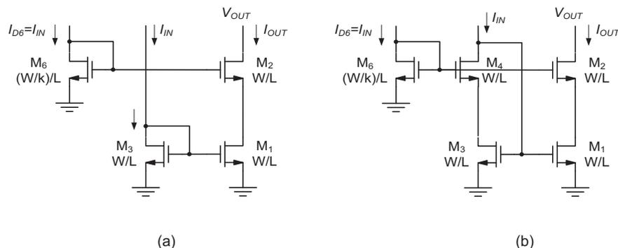
**Figure 5-16:** High-swing cascode current mirror with input branch included. (a) Non-preferred solution that suffers from a systematic mirror ratio error. (b) Solution that avoids the systematic mirror ratio error.
