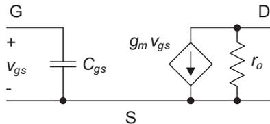
**Figure 3-6:** MOSFET small-signal model for the saturation region, including the intrinsic gate capacitance.
