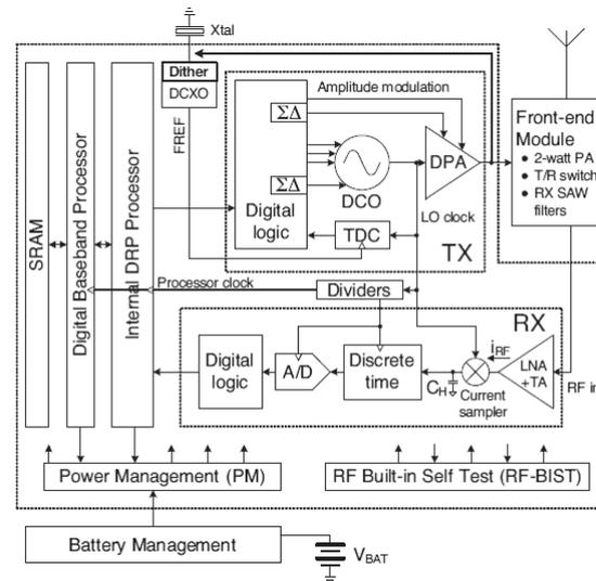
**Figure 1-2:** Block diagram of a single-chip radio (Reference 1).
