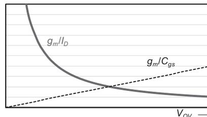
**Figure 3-8:** Tradeoff between  $g_m / I_D$  and  $g_m / C_{gs}$ .
