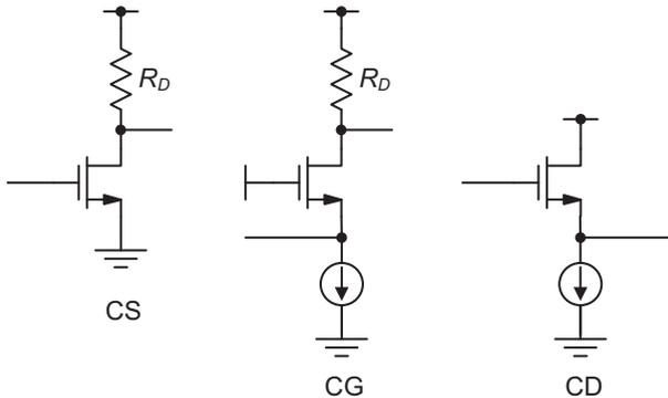
**Figure 6-1:** Amplifier configurations assumed in this section.
