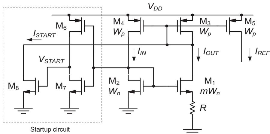
**Figure 5-21:** Complete self-biased constant- $g_m$  current reference circuit.
