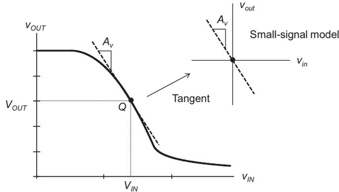
**Figure 2-10:** Concept of small-signal voltage gain. In the small signal model, the input and output voltages are linearly related through  $A_v$ , the slope of the tangent at the operating point of the large-signal transfer characteristic.
