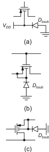
**Figure 4-4:** Connection of the well-to-substrate diode for various configurations. (a) P-channel bulk connected to the supply. (b) Bulk connected to the source in a p-channel common-gate stage. (c) Bulk connected to the source in a p-channel common-drain stage.
