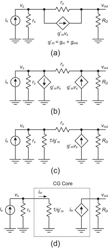
**Figure 4-10:** Modified representations of the CG small-signal circuit model. (a) Circuit with combined  $g_m$  and  $g_{mb}$  generators. (b) Split of controlled current source. (c) Representation of left side current generator using a resistor. (d) Approximate circuit model neglecting  $r_o$ .
