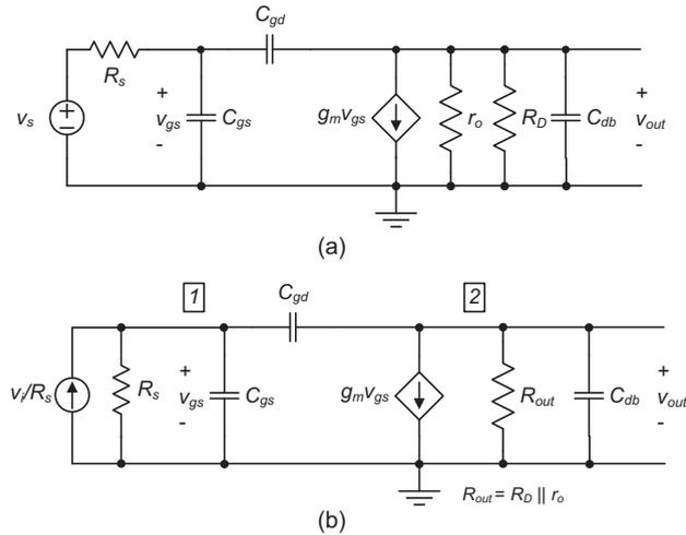
**Figure 3-13:** Small-signal model of the common-source amplifier with both intrinsic and extrinsic capacitances included. With (a) Thevenin equivalent input source configuration, and (b) Norton equivalent input source configuration.
