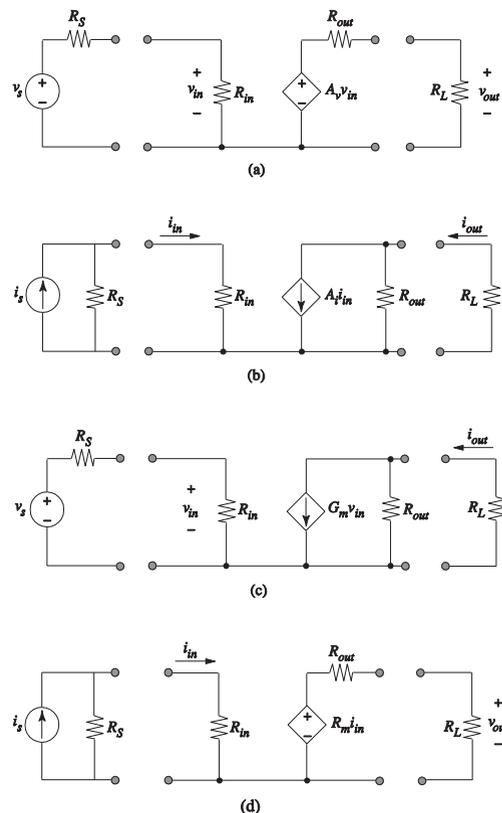
**Figure 1-9:** Two-port amplifier models with input source and load: (a) voltage amplifier, (b) current amplifier, (c) transconductance amplifier, and (d) transresistance amplifier.
