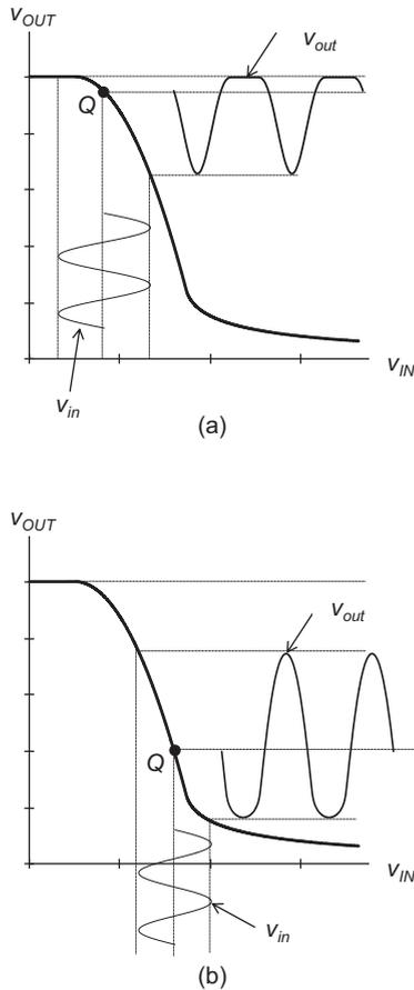
**Figure 2-11:** Examples of signal clipping and distortion. (a) Output waveform is clipped due to supply voltage limit. (b) Output waveform drives the MOSFET into the triode region.
