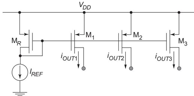
**Figure 5-9:** PMOS current mirror with multiple outputs.
