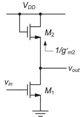
**Figure 4-29:** Common-source stage with common-gate load device.
