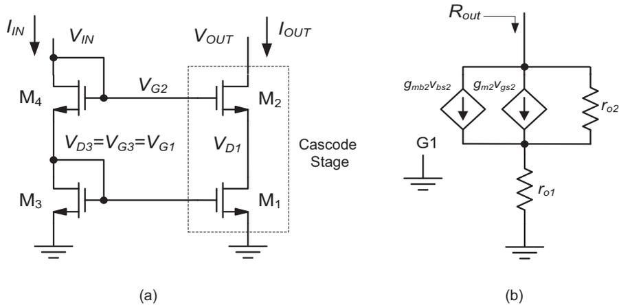
**Figure 5-11:** Basic cascode current mirror. (a) Complete circuit. (b) Small-signal circuit model for the output branch.
