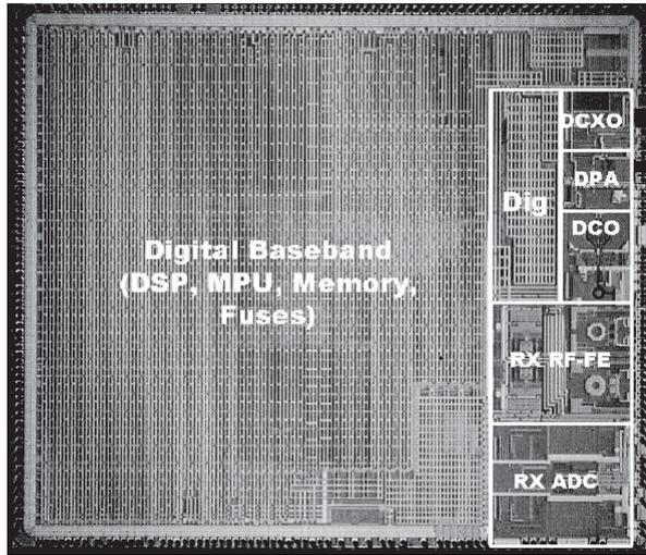
**Figure 1-3:** Chip photo of a single-chip radio (Reference 1).
