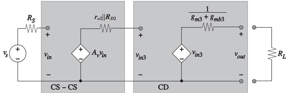
**Figure 6-3:** Small-signal model of a CS-CS-CD cascade.
