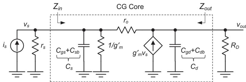
**Figure 4-13:** High-frequency small-signal model of the CG stage.
