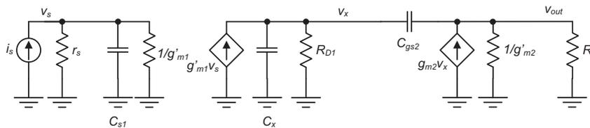
**Figure 6-7:** Simplified small-signal model of the CG-CD transresistance amplifier.
