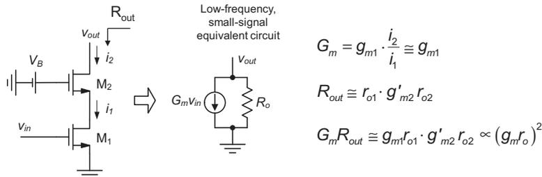
**Figure 4-26:** The cascode configuration and its low-frequency equivalent circuit.
