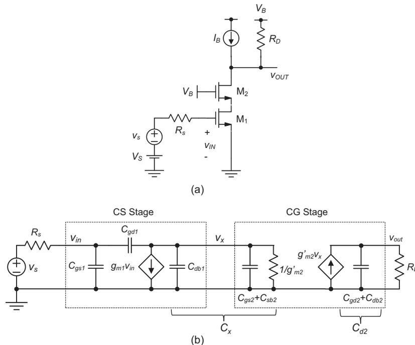
**Figure 6-8:** (a) Cascode amplifier. (b) Corresponding small-signal model.
