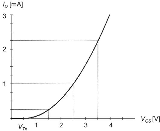
**Figure 2-5:** Plot of n-channel drain current as a function of  $V_{GS}$  (transfer characteristic). Parameters:  $V_{DS} = 5\text{ V}$ ,  $\mu_n C_{ox} = 50\ \mu\text{A/V}^2$ ,  $V_{Tn} = 0.5\text{ V}$ , and  $W/L = 10$ .
