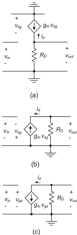
**Figure 2-15:** Small-signal model of the p-channel common-source amplifier: (a) using the p-channel model directly, (b) a flipped version of (a), and (c) with sign changes applied to show equivalence with the n-channel model.
