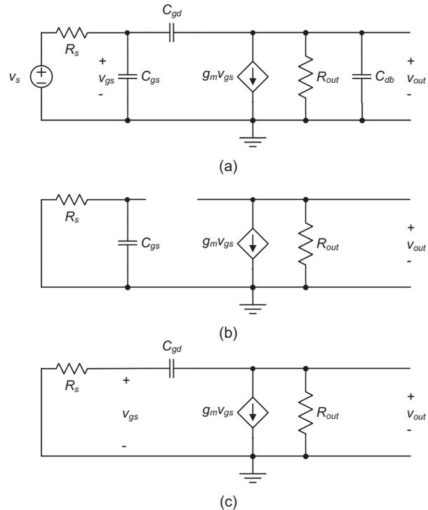
**Figure 3-18:** OCT analysis for a common-source amplifier. (a) Complete circuit. (b) Circuit for finding  $\tau_{gs}$ . (c) Circuit for finding  $\tau_{gd}$ .
