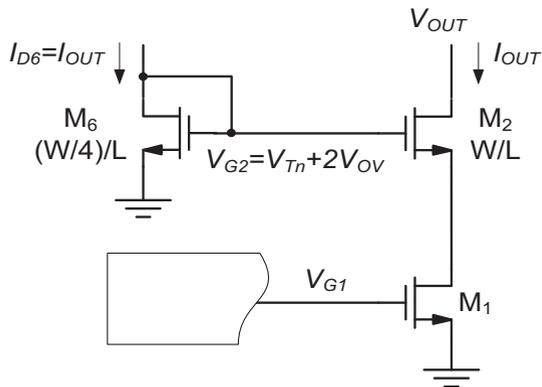
**Figure 5-15:** Basic circuit for cascode voltage generation.
