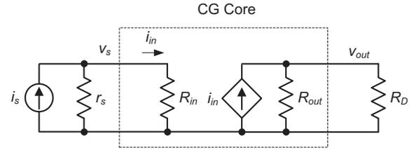
**Figure 4-12:** Small-signal unilateral two-port model of the CG stage.
