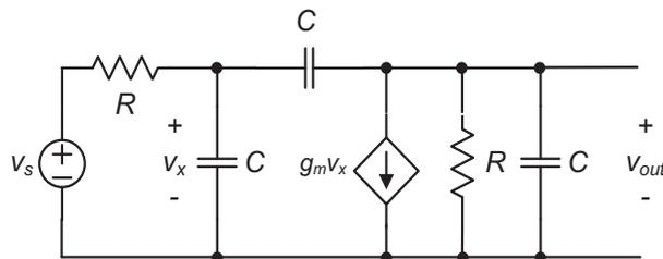
**Figure 3-21:** Circuit example with three open-circuit time constants.
