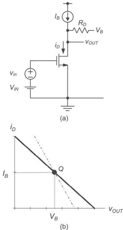
**Figure 2-19:** (a) CS amplifier with modified drain biasing scheme. (b) Load line characteristic.
