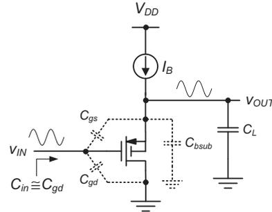
**Figure 4-22:** P-channel common-drain stage with source-bulk tie.
