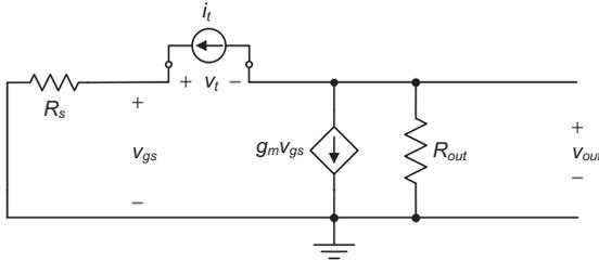
**Figure 3-19:** Circuit to determine the Thévenin resistance seen across  $C_{gd}$ .
