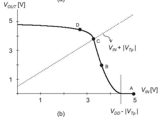
**Figure 2-14:** (a) P-channel common-source amplifier schematic. (b) Voltage transfer characteristic for  $V_{DD} = 5$  V,  $R_D = 5$  k $\Omega$ , and  $W/L = 40$ .
