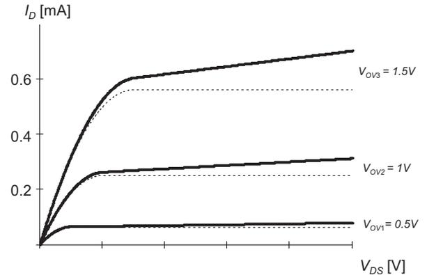
**Figure 2-21:** Realistic n-channel I-V plots, incorporating the dependence of saturation drain current on  $V_{DS}$ . (solid lines), along with the first-order model assumed previously (dotted lines). Parameters:  $W = 20 \mu\text{m}$ ,  $L = 2 \mu\text{m}$ .
