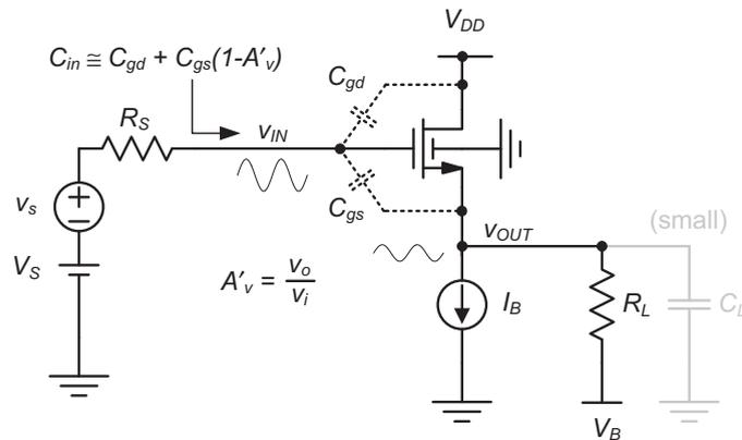
**Figure 4-21:** Circuit model for explaining the Miller effect in a common-drain stage.
