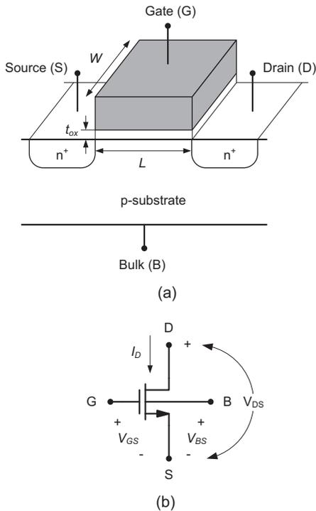
**Figure 2-1:** (a) Cross-section of an n-channel MOSFET. (b) Schematic symbol.
