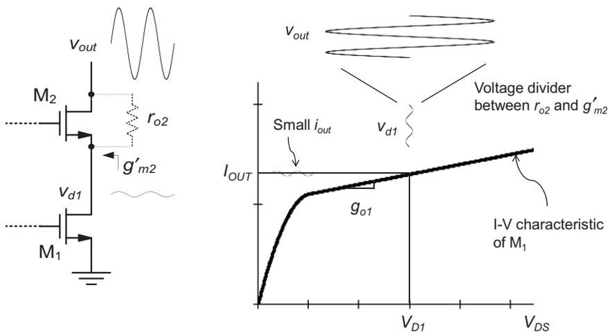
**Figure 5-12:** Qualitative inspection of the output branch in a cascode current mirror.
