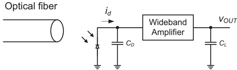
**Figure 6-11:** High-level schematic of the design problem.
