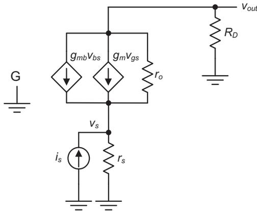
**Figure 4-9:** Low-frequency small-signal model of the CG stage.
