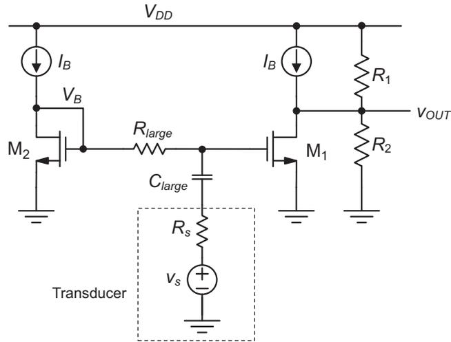
**Figure 5-23:** Replica biasing approach using AC coupling.
