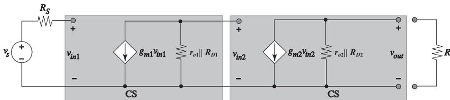
**Figure 6-2:** Small-signal model for two cascaded common-source amplifiers.
