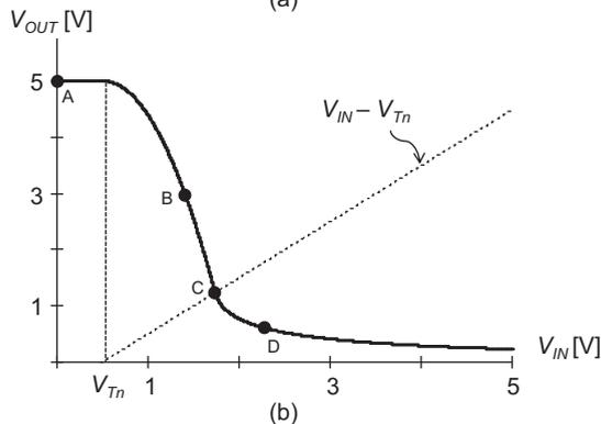
**Figure 2-7:** (a) Basic common-source amplifier schematic. (b) Voltage transfer characteristic for  $V_{DD} = 5$  V,  $R_D = 5$  k $\Omega$ , and  $W/L = 20$ .
