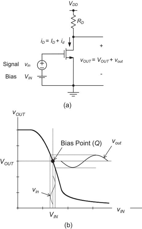
**Figure 2-9:** (a) CS amplifier with input bias. (b) Transfer characteristic showing the bias point.
