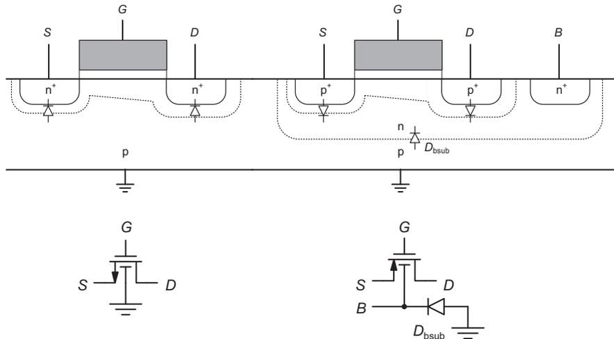
**Figure 4-2:** Cross-section of an n-well CMOS technology.
