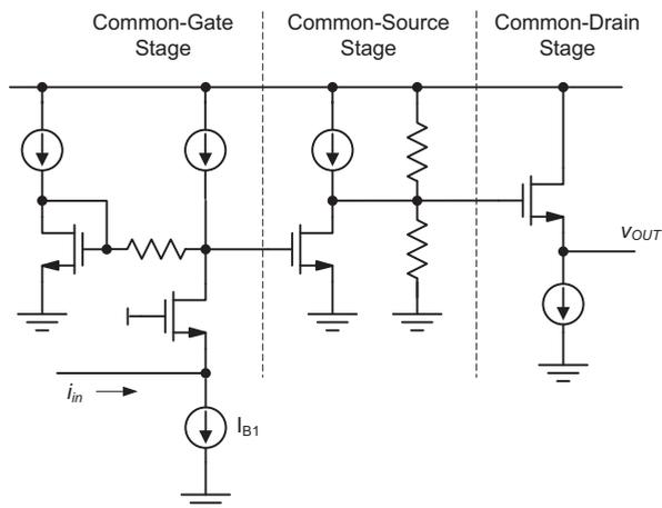
**Figure 1-5:** Example realization of a transimpedance amplifier.
