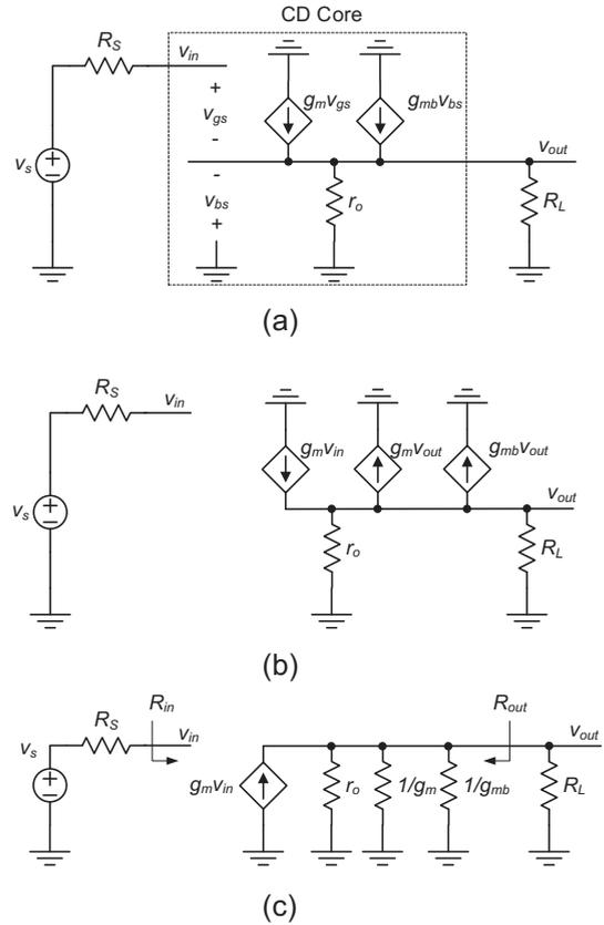
**Figure 4-17:** (a) CD small-signal, low-frequency circuit model. (b) Split of controlled current source. (c) Representation of output-controlled current generators using a resistor.
