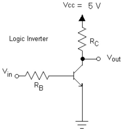
18. Determine  $V_C$  for the circuit below. Use the constant voltage drop model to find  $i_B$ . Then use load line analysis to find  $i_C$ .
