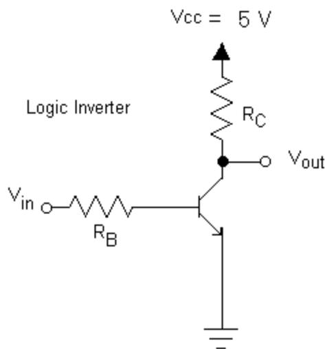
Figure 103: Logic Inverter Circuit
