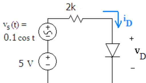
24) Determine the small signal voltage  $[v_d(t)]$  in the circuit below.
