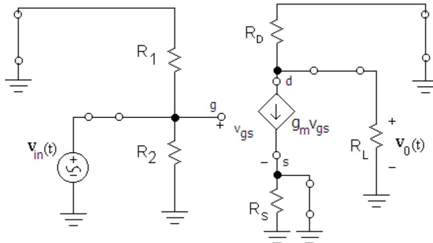
Figure 71: Small Signal Equivalent of Common Source Amplifier
