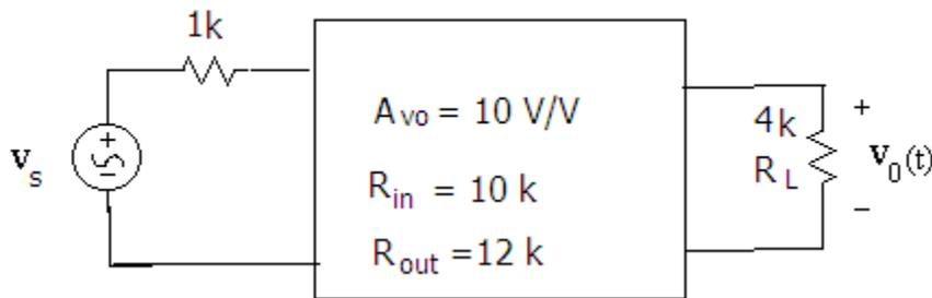
30. Find the voltage amplifier model of the circuit below (with the load removed) by determining the small signal parameters of voltage gain ( $A_{vo}$ ), input resistance ( $R_{in}$ ), and output resistance ( $R_{out}$ ). Using this model, find the voltage gain of the circuit with the load attached. Assume  $K_n=1$  mA/V<sup>2</sup>, and  $V_{Th}=1$  V. Note that there is no bypass capacitor across the source resistance! Otherwise, this is the same circuit as that in problem 26.
