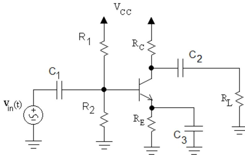
Figure 109: Common Emitter Amplifier Circuit
