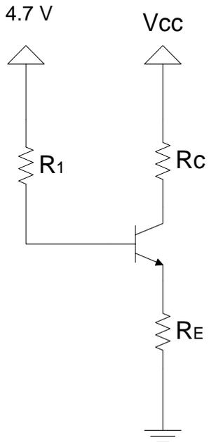
17. Draw the transfer characteristic graph showing  $v_{out}$  vs  $v_{in}$  for the inverter circuit below for  $V_{in}$  from 0 to 5 V. Drawing a single graph, include plots for  $R_C=2\text{ k}\Omega$ ,  $10\text{ k}\Omega$ , and  $50\text{ k}\Omega$ . Assume  $\beta=100$  and  $R_B=100\text{ k}\Omega$ . Judging from your graph, do any of these values for  $R_C$  seem unreasonable for a logic inverter?
