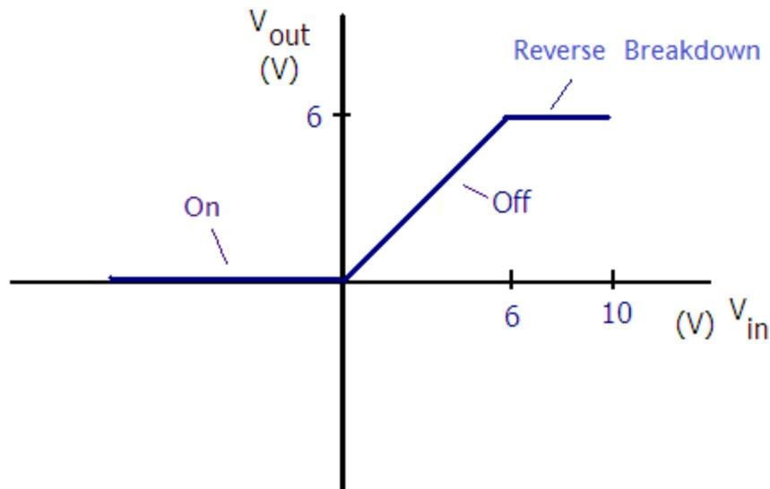
Figure 24: Transfer Characteristics of a Clipper Circuit with One Diode
