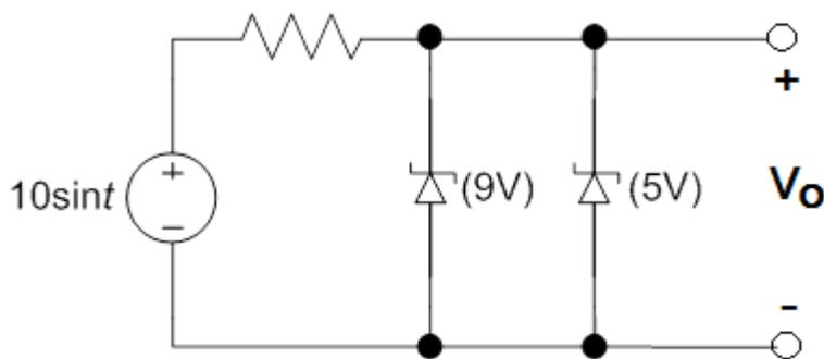
16) Draw the output voltage waveform for the following circuit. Assume the constant voltage drop model for the junction diodes.
