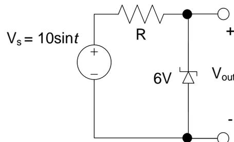
Figure 22: Simple Clipper Circuit
