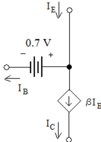
Figure 99: PNP Active Mode Circuit Model
