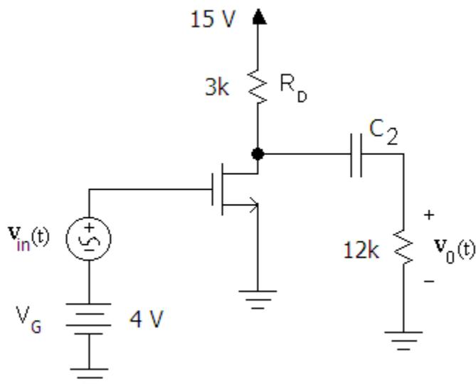
18. Determine the small signal output resistance of the circuit above. Assume  $K_n=1\text{mA/V}^2$ , and  $V_{Th}=1\text{V}$ .
