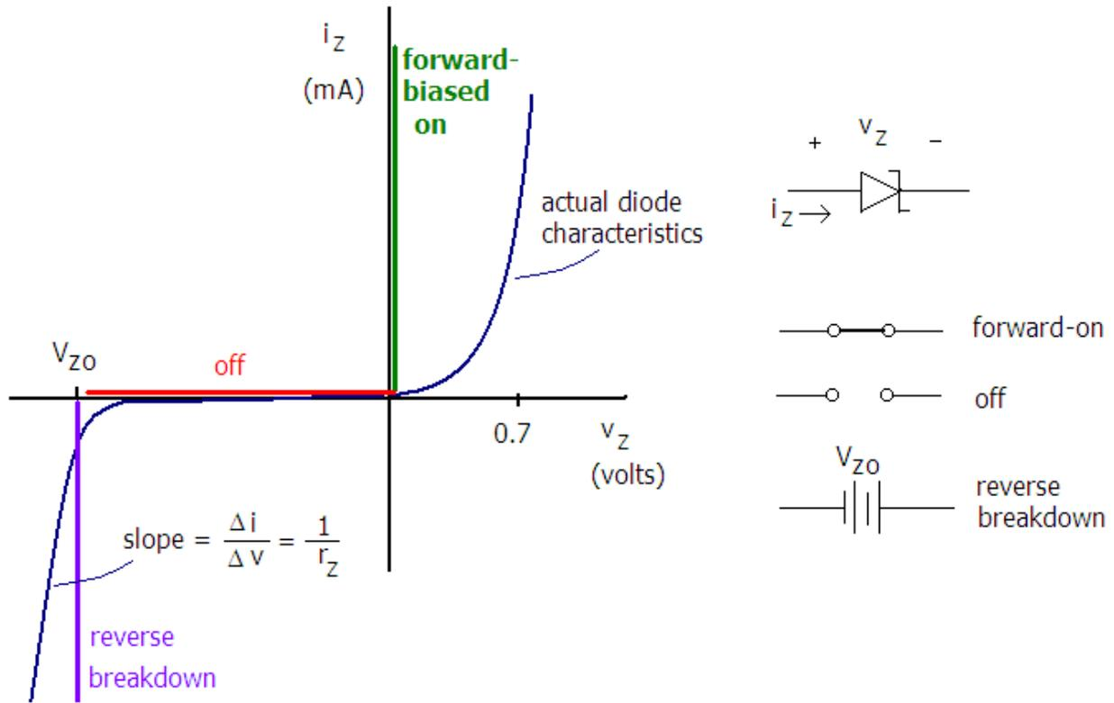
Figure 21: Zener Diode I-V Characteristic Curve and Models
