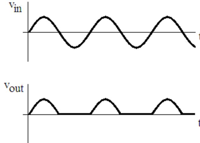
Figure 18: Half Wave Rectifier Input/Output Waveforms
