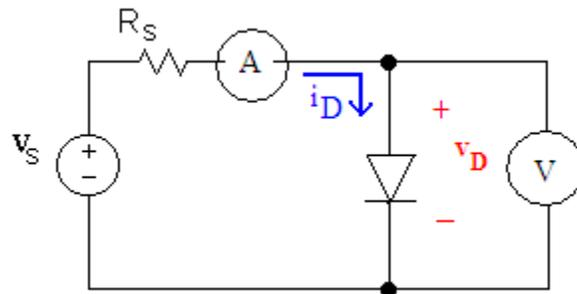
Figure 11: Circuit to Illustrate I-V Characteristic of a Junction Diode
