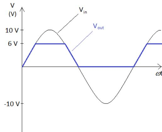
Figure 23: Clipper Circuit Input/Output Waveforms
