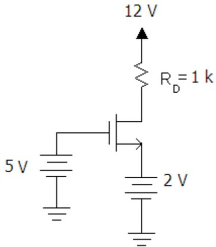
10. Find  $I_D$  and  $V_{DS}$  for the circuit shown below. The NMOS parameters are  $V_{Th}=1\text{ V}$  and  $K_n=0.25\text{ mA/V}^2$ .
