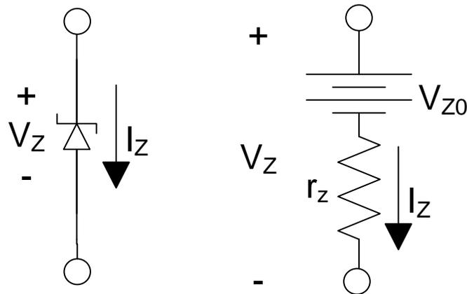
Figure 28: Battery Plus Resistance Model for Zener
