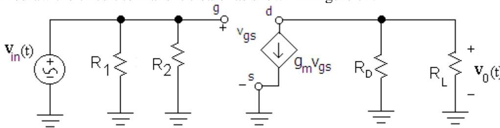
Figure 72: Simplified Small Signal Equivalent of Common Source Amplifier
