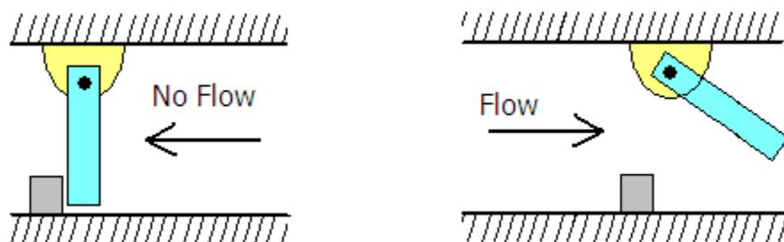
Figure 10: Check Valve Illustration
