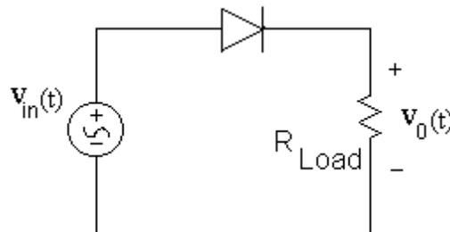
Figure 17: Half Wave Rectifier
