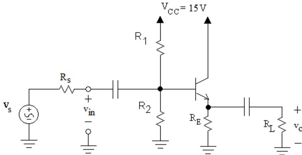
32. Determine  $A_v$  and  $A_i$  for the emitter follower amplifier shown below. Assume that  $\beta=100$ ,  $V_T=25$  mV,  $R_1=R_2=5$  k $\Omega$  and  $R_E=R_L=1$  k $\Omega$ . If you have done problem 31, you can use those results to help solve this problem.
