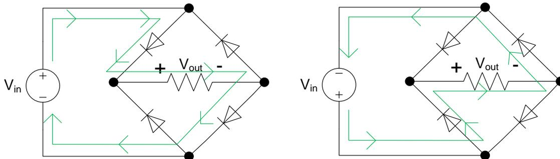
Figure 19: Full Wave Rectifier
