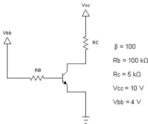
5. Determine all transistor terminal voltages ( $V_B$ ,  $V_C$ , and  $V_E$ ) and currents ( $I_B$ ,  $I_C$ , and  $I_E$ ) for the circuit below.
