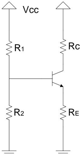
20. Determine all terminal voltages and currents for the circuit below. Assume the following component values:  $V_{CC}=20\text{ V}$ ,  $R_1=40\text{ k}\Omega$ ,  $R_2=60\text{ k}\Omega$ ,  $R_C=1\text{ k}\Omega$ ,  $R_E=1\text{ k}\Omega$ , and  $\beta=100$ .
