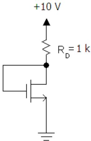
12. Design the circuit so that  $I_D = 10\text{ mA}$ . The NMOS parameters are  $V_{Th} = 1\text{ V}$  and  $K_n = 0.25\text{ mA/V}^2$ .
