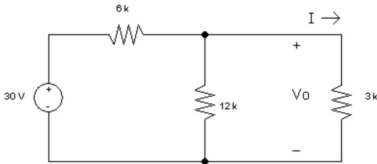
5. Redraw the circuit below so that it is in the “electronics” format. Take the ground reference to be at the bottom of the schematic.
