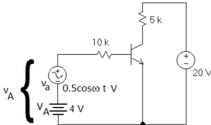
Figure 7: Amplifier Showing DC bias voltage and AC signal voltage
