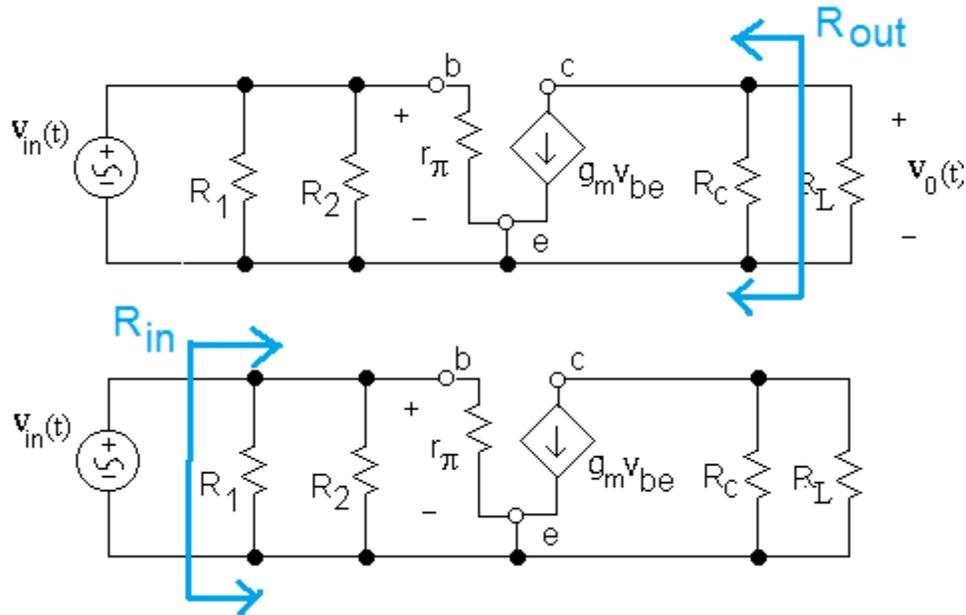
Figure 110:  $R_{in}$  and  $R_{out}$  Parameters for Common Emitter Amplifier
