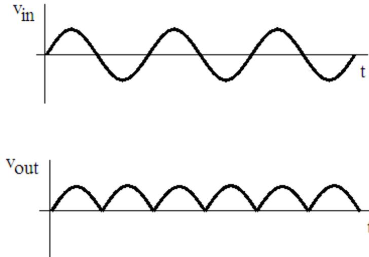
Figure 20: Full Wave Rectifier Input/Output Waveforms
