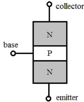
Figure 89: Physical Construction of an NPN Transistor
