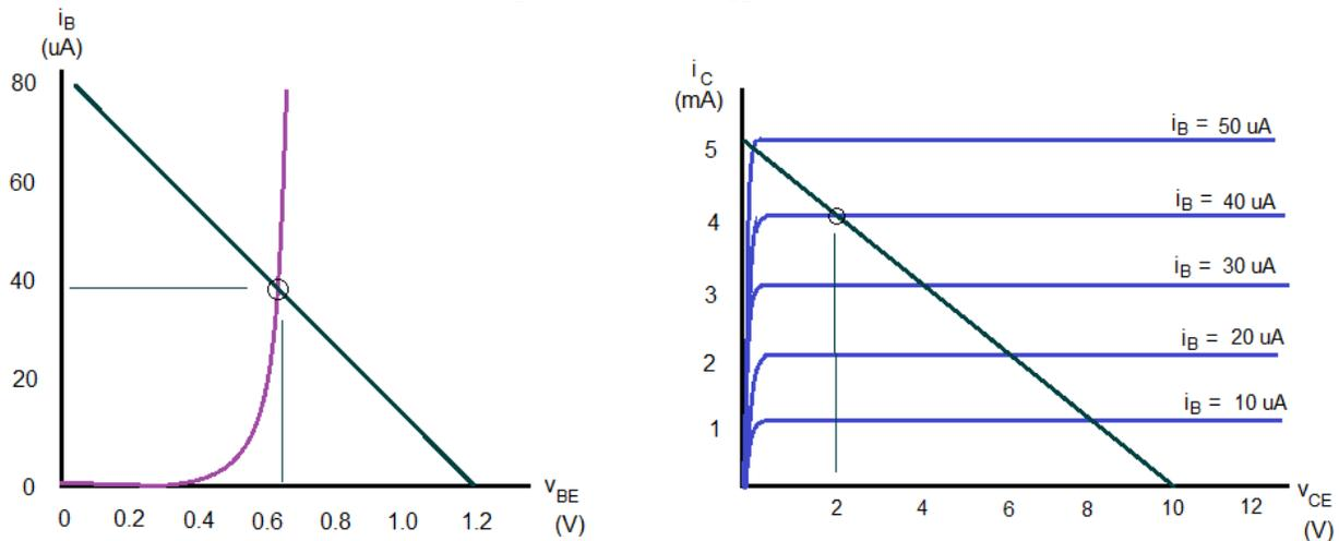
Figure 102: Load Line Characteristic Curves
