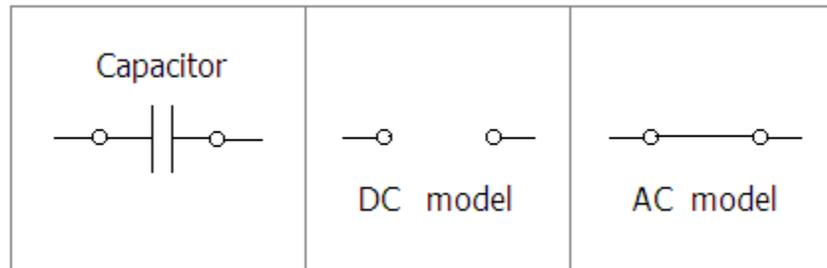
Figure 67: DC and AC Capacitor Models
