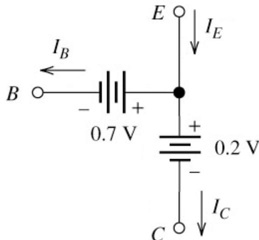
Figure 100: PNP Triode Circuit Model
