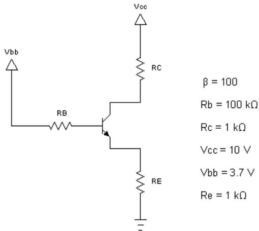
8. Determine all transistor terminal voltages ( $V_B$ ,  $V_C$ , and  $V_E$ ) and currents ( $I_B$ ,  $I_C$ , and  $I_E$ ) for the circuit below. Note that the value of  $\beta$  is 1000!
