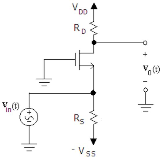
27. Derive the expressions for  $A_{VO}$ ,  $R_{in}$ , and  $R_{out}$  for the “common gate amplifier” shown above. Derive the expression in terms of  $g_m$  and the labeled resistors.
