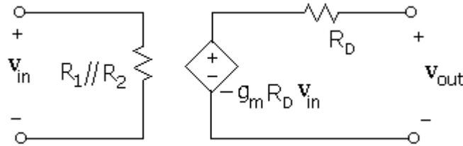
Figure 82: Voltage Amplifier Model of a Common Source Amplifier
