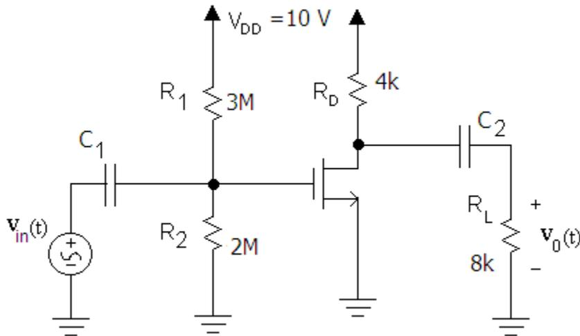
22. Determine the small signal  $R_{in}$  and  $R_{out}$  for the amplifier above.
