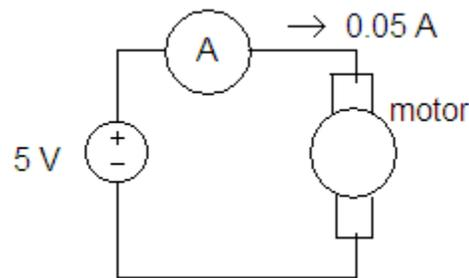
There are 2 designs that we will investigate to supply the 5 V to the motor; a voltage divider circuit and a regulator using a zener diode. We begin with the voltage divider design shown below.
