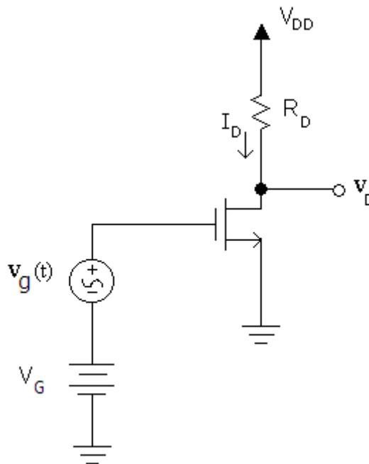
Figure 57: Conceptual Amplifier Circuit
