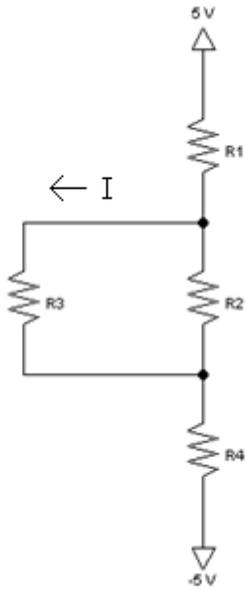
4. Redraw the circuit below so that it is in the “electronics” format. Clearly indicate  $V_0$  and  $I$  on your schematic. Take the ground reference to be at the bottom of the schematic.
