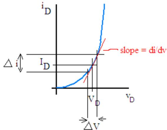
Figure 33: Small Signal Analysis - Slope at Q Point
