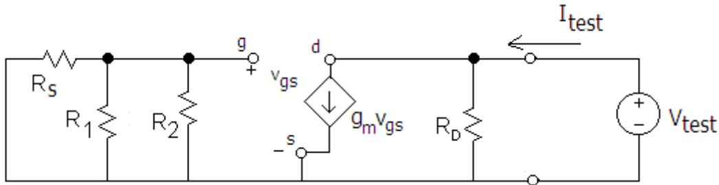
Figure 80: Circuit to Determine  $R_{out}$
