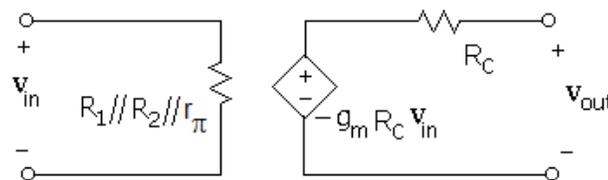
Figure 113: Voltage Amplifier Model of Common Emitter Amplifier
