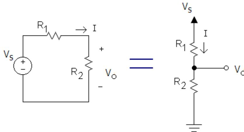
Figure 5: Schematic Conversion Example
