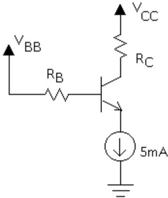
10. Determine all transistor terminal voltages ( $V_B$ ,  $V_C$ , and  $V_E$ ) and currents ( $I_B$ ,  $I_C$ , and  $I_E$ ) for the circuit below.
