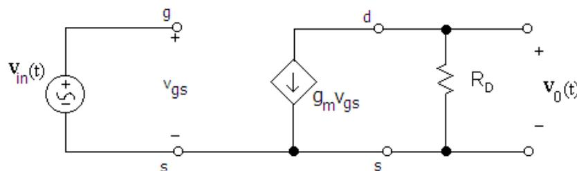
Figure 65: Simplified Small Signal Equivalent
