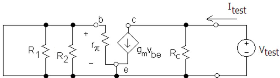
Figure 111: Determining  $R_{out}$
