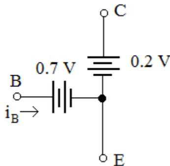
Figure 98: Saturation Model
