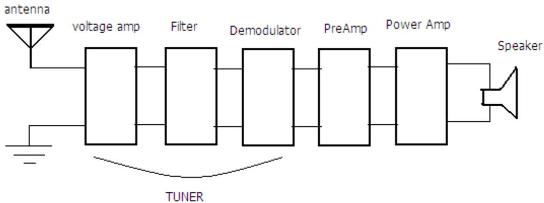
Figure 3: Block Diagram of a Radio
