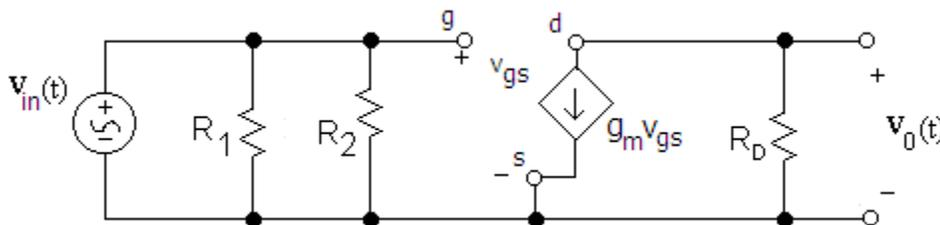
Figure 81: Finding  $A_{vO}$  for a Common Source Amplifier
