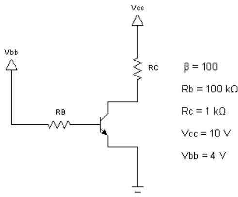
6. Determine all transistor terminal voltages ( $V_B$ ,  $V_C$ , and  $V_E$ ) and currents ( $I_B$ ,  $I_C$ , and  $I_E$ ) for the circuit below.
