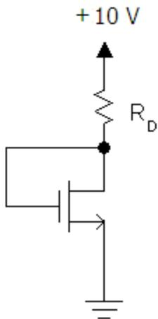
13. For the PMOS transistor below, assume that  $V_{Th} = -0.75\text{ V}$ . Determine the following:
