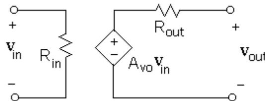
Figure 77: Voltage Amplifier Model
