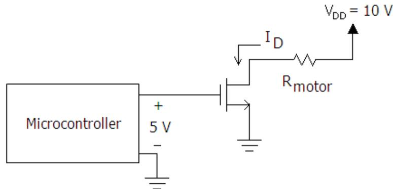
Figure 51: MOSFET as Switch
