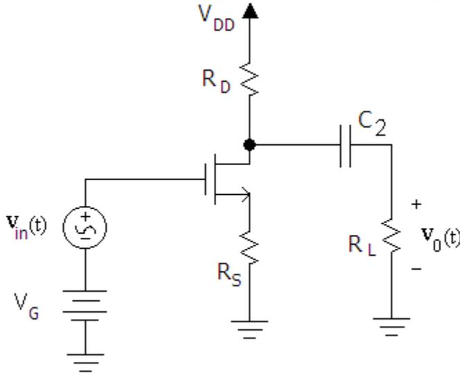
20. Determine the voltage gain of the circuit below. Assume  $K_n=1\text{mA/V}^2$ , and  $V_{Th}=1\text{V}$ .
