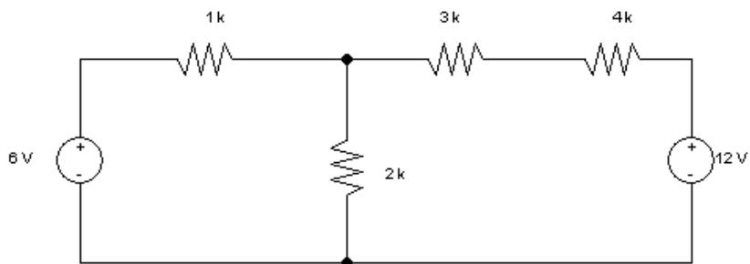
6. Redraw the circuit below so that it is in the “electronics” format. Clearly indicate  $I$  on your schematic.
