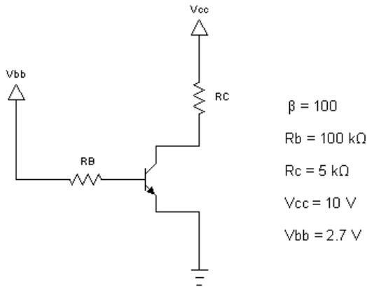
7. Determine all transistor terminal voltages ( $V_B$ ,  $V_C$ , and  $V_E$ ) and currents ( $I_B$ ,  $I_C$ , and  $I_E$ ) for the circuit below.
