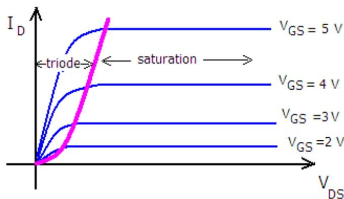
Figure 48:  $I_D$  vs.  $V_{DS}$  Curves for various  $V_{GS}$
