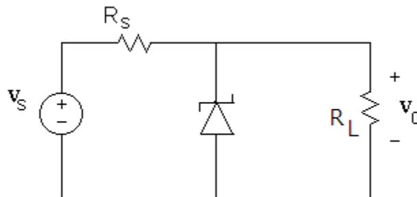
Figure 25: Zener Shunt Voltage Regulator
