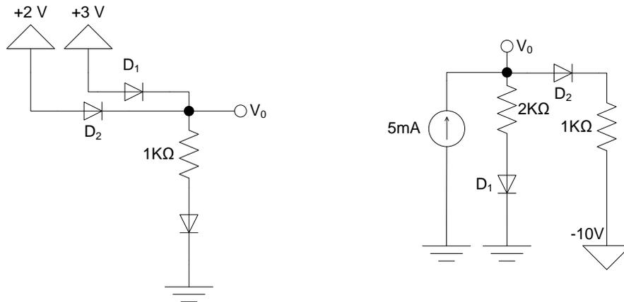
5) Determine the voltage  $V_0$  using the constant voltage drop model.
