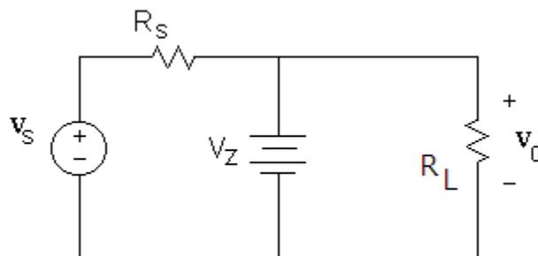
Figure 26: Regulator with Zener Modeled as a Voltage Source
