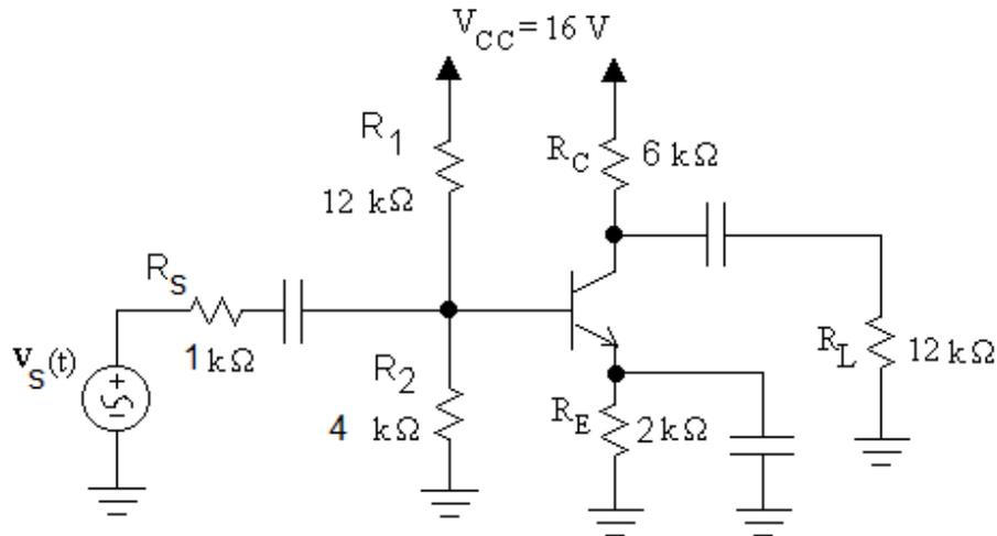
Figure 114: Common Emitter Amplifier with Circuit Parameter Values
