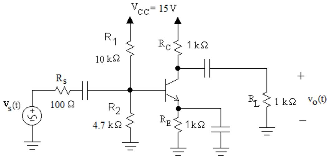
29. Determine  $A_{vo}$ ,  $R_{in}$ ,  $R_o$  for the amplifier below. Draw the voltage amplifier model for this circuit. Assume  $\beta = 100$  and  $V_T = 25$  mV.
