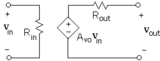
Figure 108: Voltage Amplifier Model
