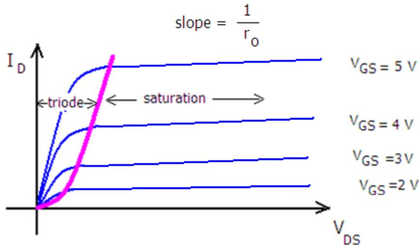
Figure 84: Effect of  $V_{DS}$  on  $I_D$  in Saturation
