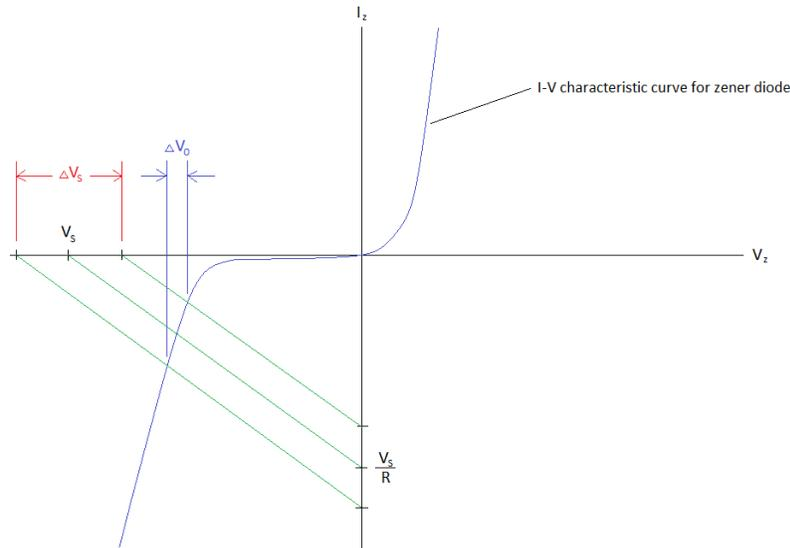
Figure 30: Load Lines for Voltage Regulator
