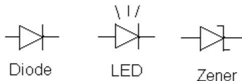
Figure 9: Schematic Symbols for Diodes
