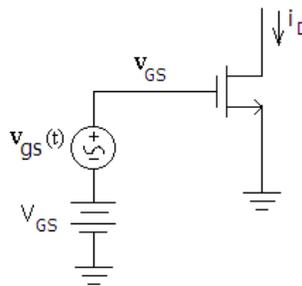
Figure 61: Small Signal in Series with Gate Bias Voltage
