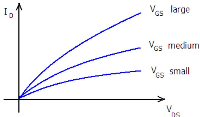
Figure 45:  $I_D$  vs.  $V_{DS}$  Characteristic for Various Fixed  $V_{GS}$
