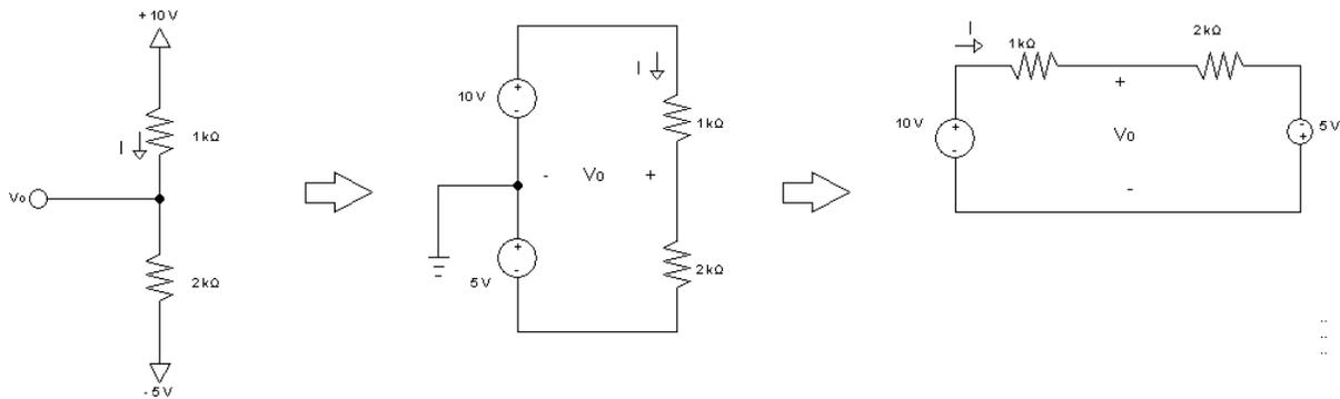
Figure 6: Schematic with Positive and Negative Voltage Sources
