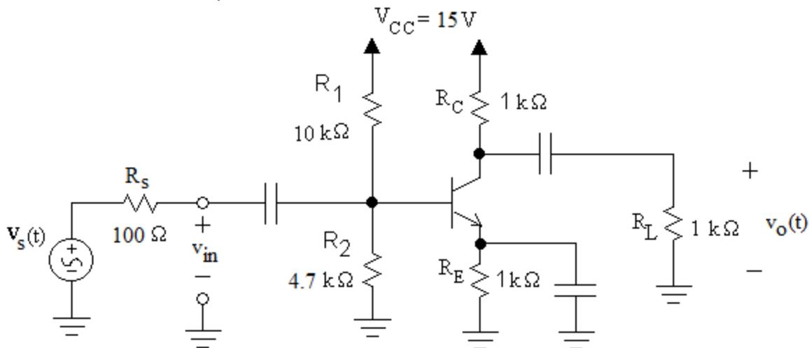
30. Using voltage amplifier model you determined in problem 29, determine  $A_v$  and  $A_i$  for this circuit with the source and load resistors shown.
