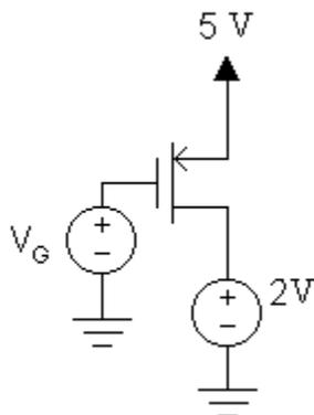
14. For the PMOS circuits below, find the desired parameter. Assume  $K_P=0.1 \text{ mA/V}^2$  and  $V_{Th}=-1\text{V}$ .
