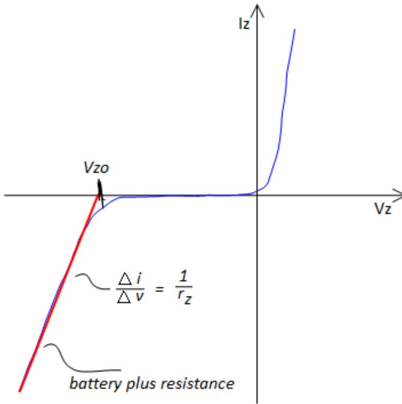
Figure 27: Zener I-V Characteristics Showing Incremental Resistance
