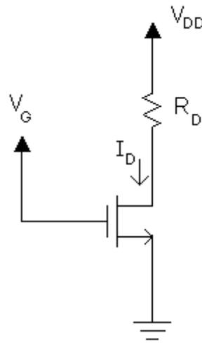
Figure 49: MOSFET Circuit to Investigate Load Line Analysis
