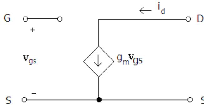
Figure 63: MOSFET Small Signal Model
