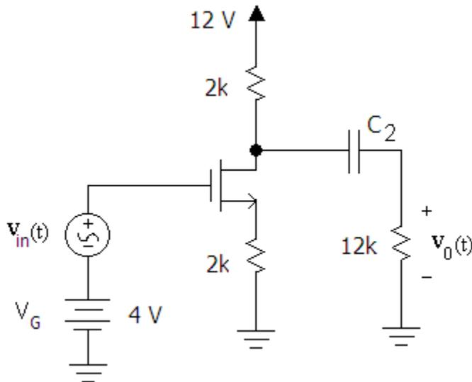
21. Determine the small signal voltage gain of the following circuit. Assume  $V_{Th}=2\text{V}$  and  $K_n=0.25\text{mA/V}^2$ .
