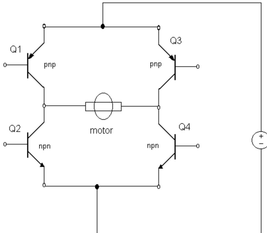
Figure 104: H Bridge Motor Control Circuit
