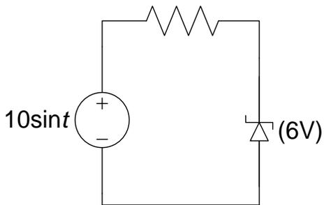
15) Draw the output voltage waveform for the clipper circuit below.
