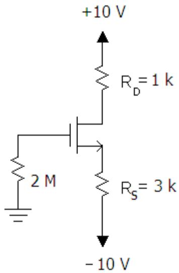
11. Find  $I_D$  and  $V_{DS}$  for the circuit shown below. The NMOS parameters are  $V_{Th}=1\text{ V}$  and  $K_n=0.25\text{ mA/V}^2$ .
