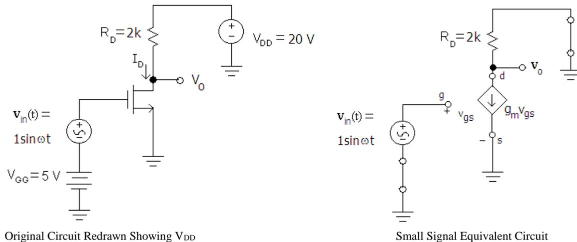
Figure 64: Construction of Small Signal Equivalent Circuit
