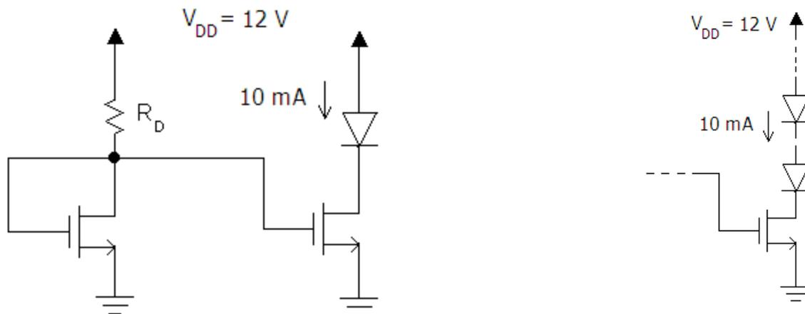
17. Determine the small signal voltage gain of the circuit below. Assume  $K_n=0.5\text{ mA/V}^2$ , and  $V_{Th}=2\text{V}$ .
