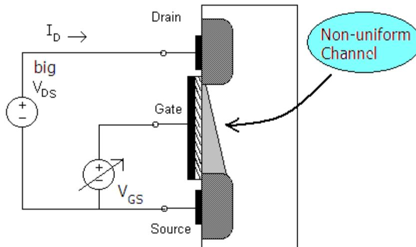
Figure 46: MOSFET in Saturation
