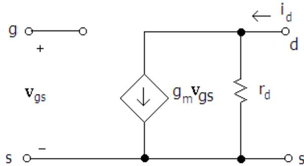
Figure 85: Small Signal Model Including  $r_d$ .
