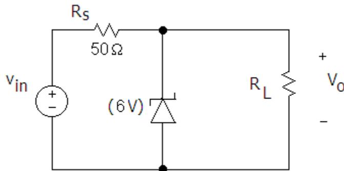
27) Design a  $5\text{ V}$  zener voltage regulator that operates from a voltage source that varies from  $8$  to  $10\text{ V}$ . The load current varies from  $0$  to  $20\text{ mA}$ .
