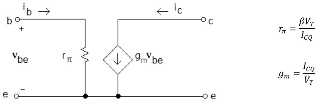
Figure 106: BJT Small Signal Model Using  $g_m$
