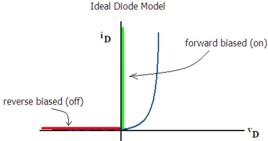
Figure 14: Ideal Diode I-V Characteristic
