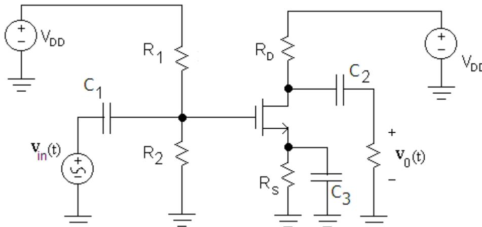
Figure 70: Common Source Amplifier with Voltage Sources Drawn
