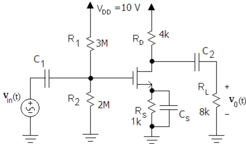
29. If an amplifier with voltage amplifier parameters of  $A_{vo}=10$  V/V,  $R_{in}=10$  k, and  $R_{out}=12$  k is connected to the circuit below, determine the voltage gain of the circuit  $A_v=v_o/v_s$ .
