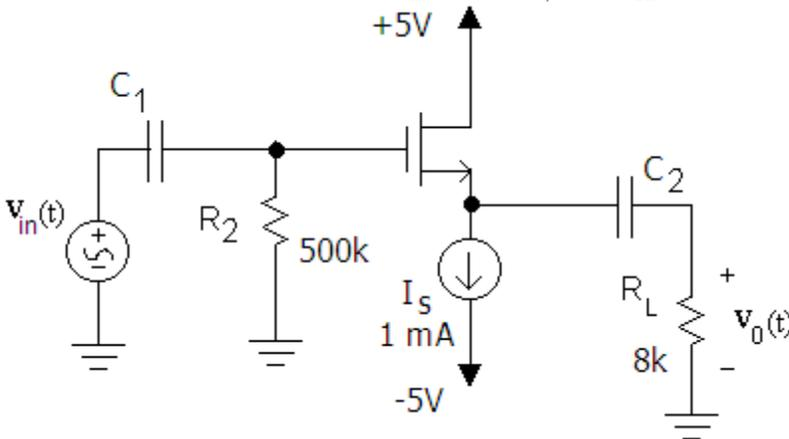
25. Determine the small signal parameters of voltage gain, input resistance and output resistance of the following circuit. Assume  $K_n=0.2 \text{ mA/V}^2$ , and  $V_{Th}=1V$ .
