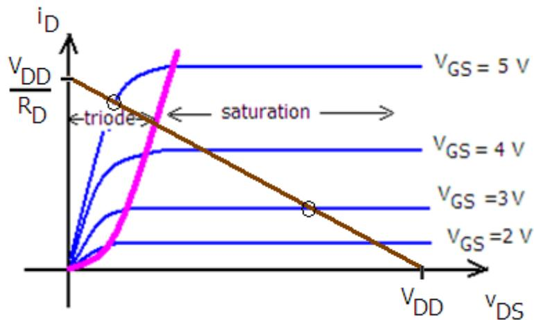
Figure 50: Load Line on Characteristic Curves
