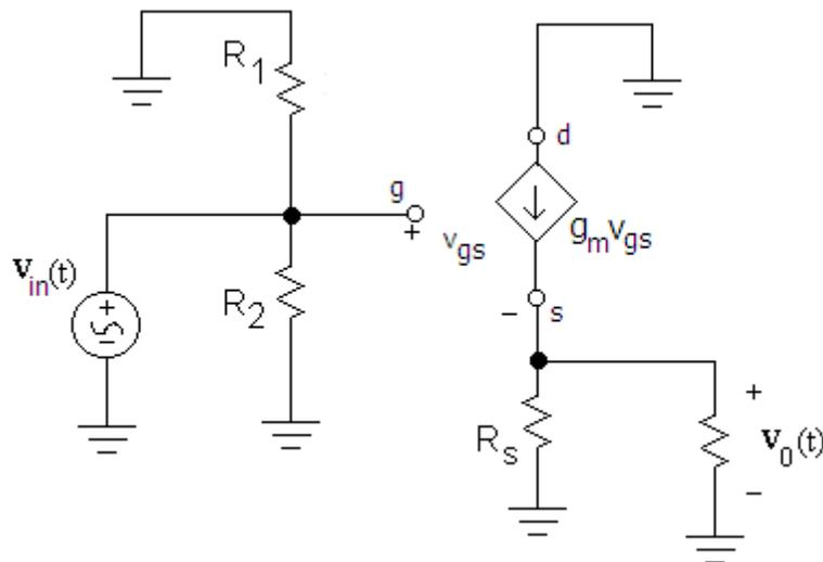
Figure 74: Small Signal Equivalent of Source Follower
