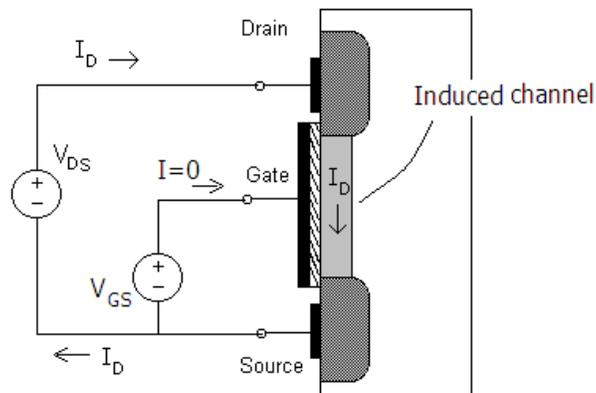
Figure 40: MOSFET with Induced Channel
