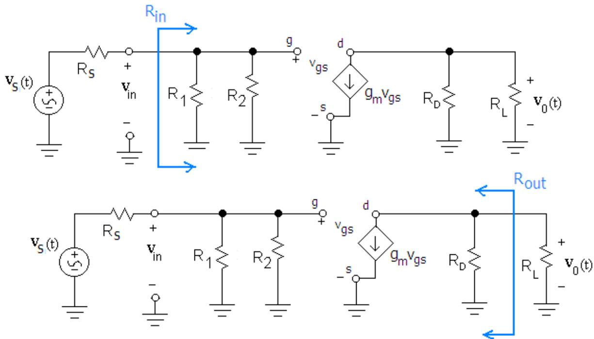
Figure 79: Small Signal Input and Output Resistances
