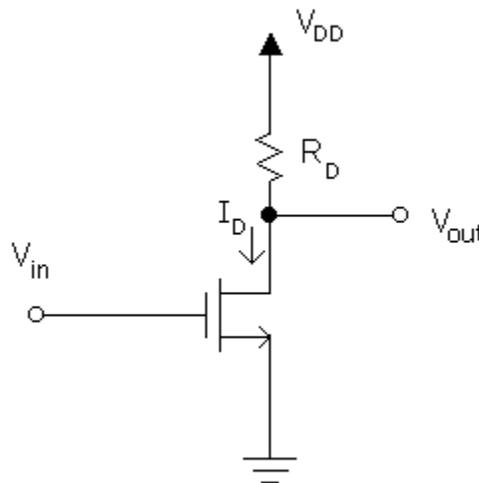
Figure 53: Logic Inverter
