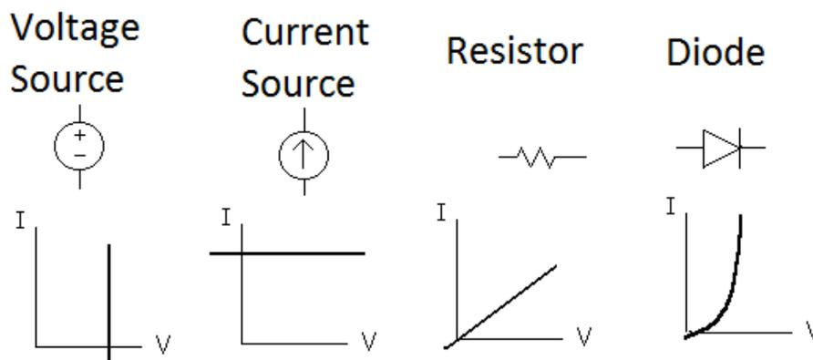
Figure 4: I-V Characteristics of Various Circuit Elements
