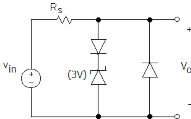
19) The solar panel is to be used to charge the 12V battery. The solar panel will produce a voltage between 18 V at full sun to 0 V at dark. Design a circuit that can be used to charge the 12 battery using a junction diode, a zener diode, and resistor(s).
