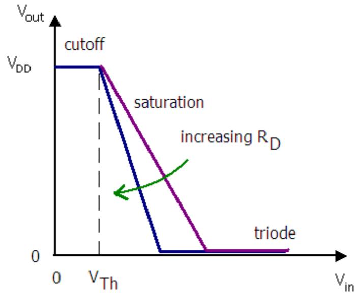
Figure 54: Inverter Transfer Characteristic
