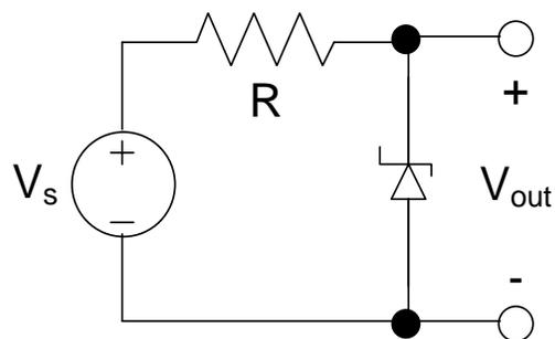
Figure 29: Shunt Regulator with Load of Infinite Resistance
