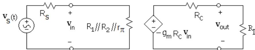
Figure 115: Terminated Voltage Amplifier Model of Common Emitter Amplifier
