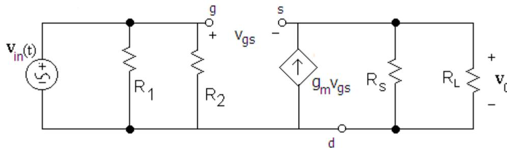
Figure 75: Small Signal Equivalent of Source Follower Simplified
