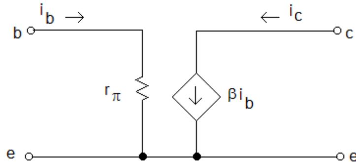
Figure 107: BJT Small Signal Model Using Beta
