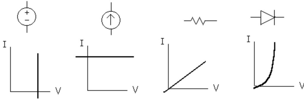
Figure 13: I-V Characteristics of Various Circuit Elements
