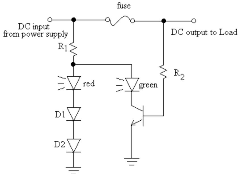
24. If the DC input voltage from the power supply is 5 V, select  $R_1$  and  $R_2$  so that the current flow through the LEDs is limited to approximately 20 mA. A current of 5 mA is sufficient to turn on either LED. Assume  $\beta=200$ .
