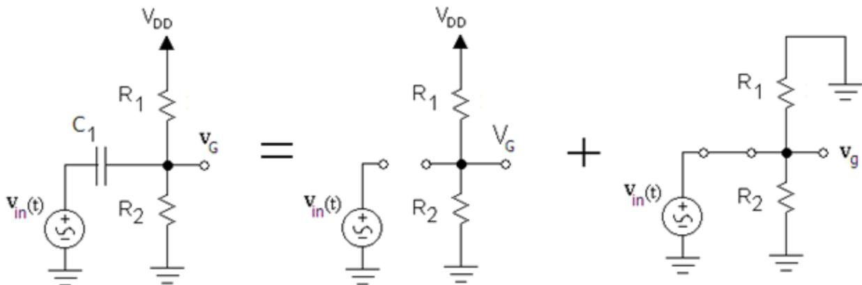
Figure 68: Capacitor AC and DC models
