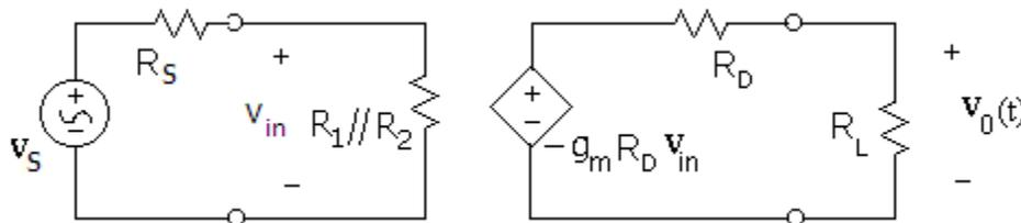
Figure 83: Voltage Amplifier Model with Source and Load Attached
