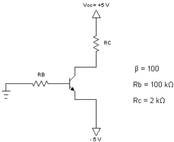
11. Determine all transistor terminal voltages ( $V_B$ ,  $V_C$ , and  $V_E$ ) and currents ( $I_B$ ,  $I_C$ , and  $I_E$ ) for the circuit below.
