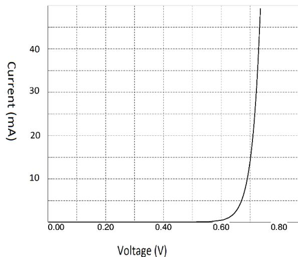
Figure 12: Diode I-V Characteristic Curve
