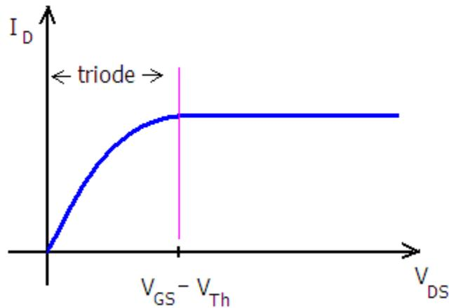
Figure 44: MOSFET  $I_D$  vs.  $V_{DS}$  for a Single Fixed  $V_{GS}$
