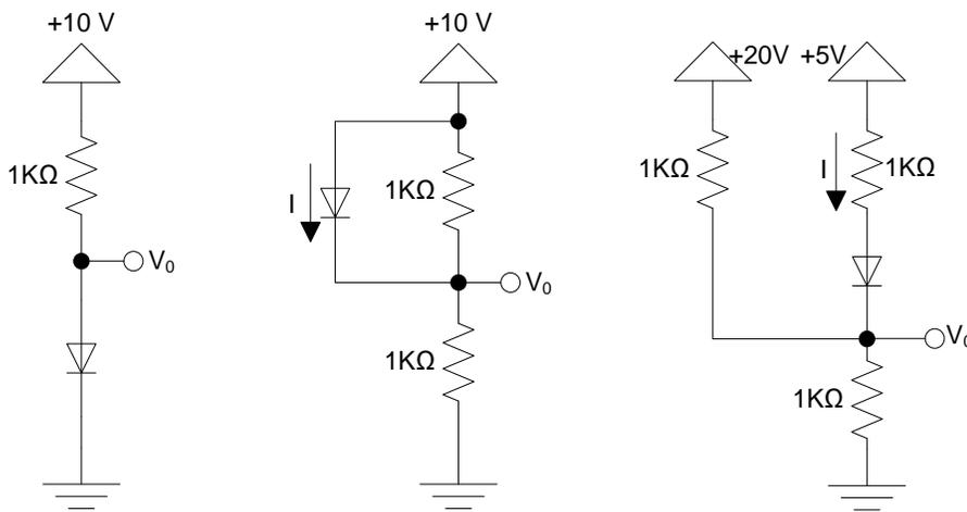
6) For the circuits below, determine the voltage  $V_0$  using the constant voltage drop model.
