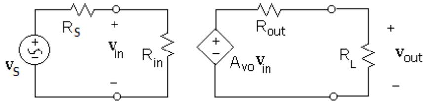
Figure 78: Voltage Amplifier Model Terminated with Source and Load
