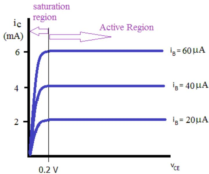
Figure 96:  $i_C$  vs.  $v_{CE}$  Curves for Several Base Currents
