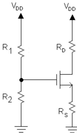
Figure 66: Four Resistor Bias Circuit
