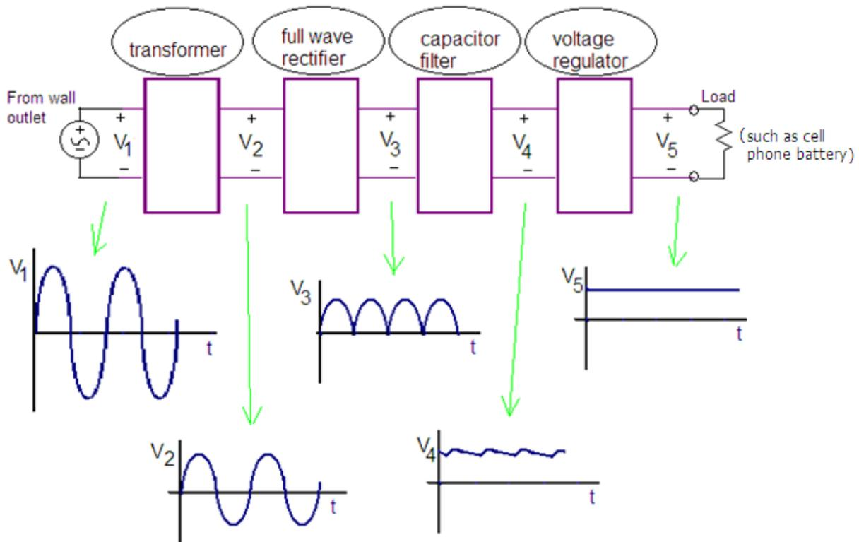
Figure 2: AC to DC Conversion Block Diagram
