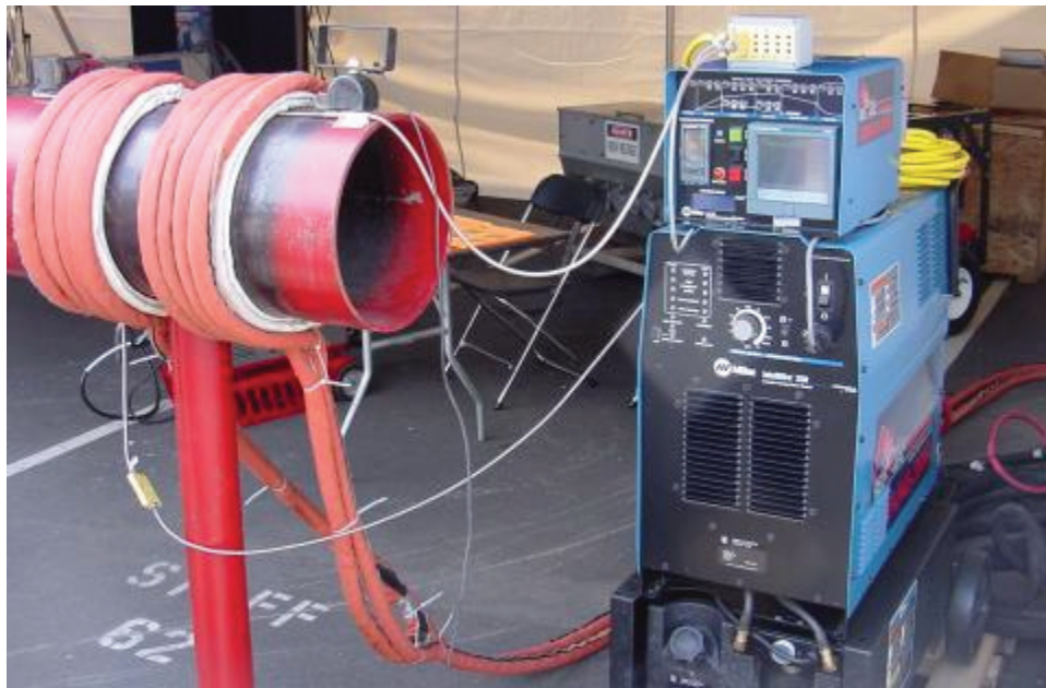
Figure 8.31 Induction heating: Primary insulated winding induces current into lossy iron pipe (secondary).
