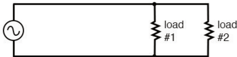
Figure 4.17 Single phase power system schematic diagram shows little about the wiring of a practical power circuit.
