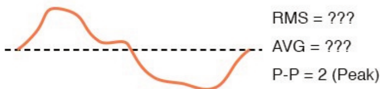
Figure 4.16 Arbitrary waveforms have no simple conversions.
