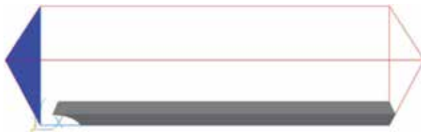
Figure 1. The plane of inlet boundary conditions specification.
