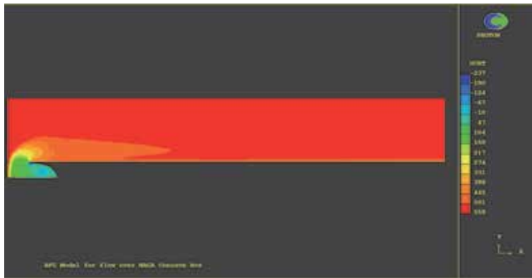
Figure 11. Contour plot of the velocity distribution on the computational field for the modified simulation ( k-\epsilon hybrid).
