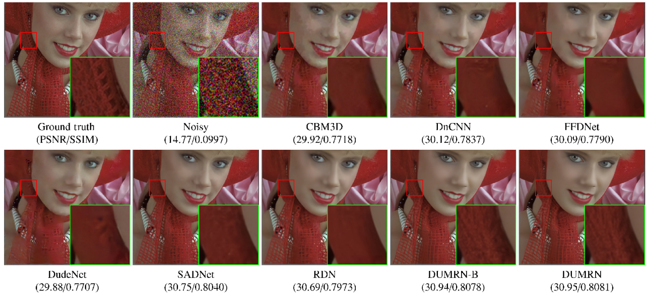
Fig. 4 Color image denoising results on image kodim04 from Kodak24 with noise level \sigma = 50 .
