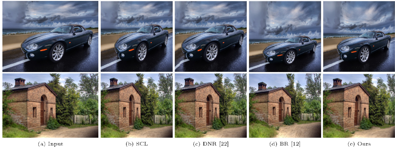
Fig. 9 Results of the proposed warping method and manual interactive methods when resizing images to 75% of their original width. (a) Input. (b) Linear scaling result. (c) Result using DNR. (d) Result using BR [12]. (e) Our result using 50 elements (approx. 460 DOFs).
