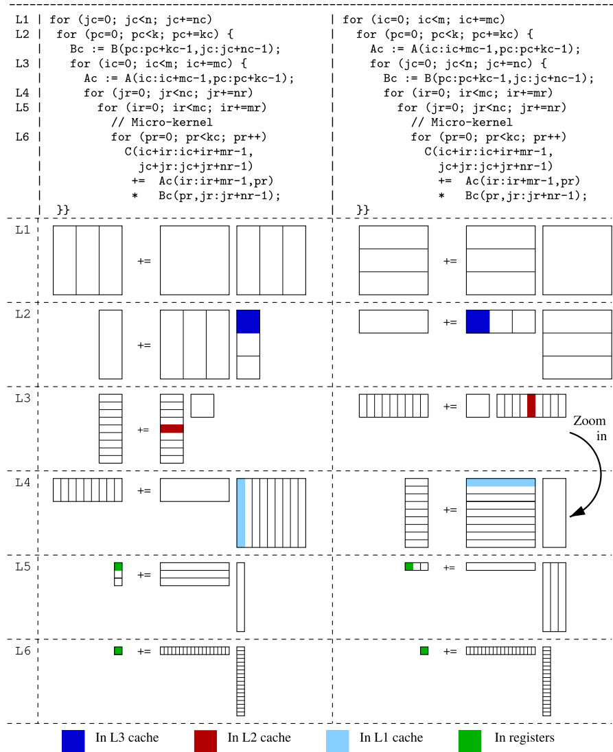
Fig. 1 Variants of the BLIS family for GEMM with C streamed from memory into the processor registers: B3A2C0 (left) and A3B2C0 (right)
