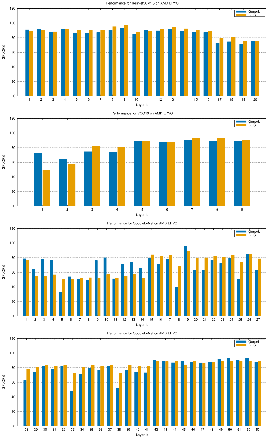
Fig. 8 Performance of the best algorithm+micro-kernel on AMD EPYC 7282
