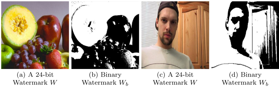
Fig. 3 The watermark images used in the experiments. Each binary watermark is the most significant bitplane of the grayscale image of its color image counterpart
