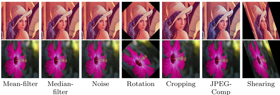
Fig. 6 Attacks on watermarked Leena (from SIPI) and Flower image (from MSRA dataset)
