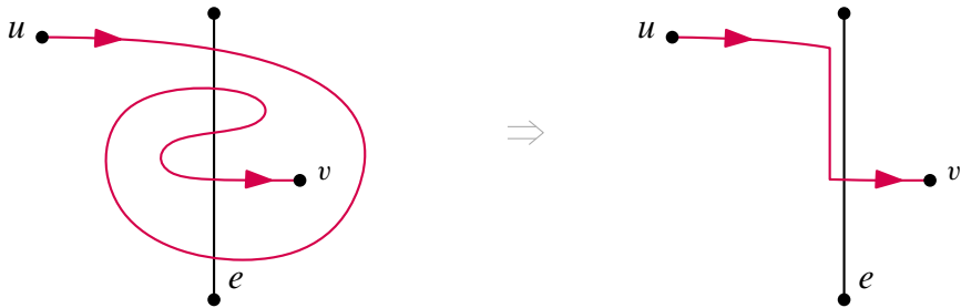
Fig. 14 Rerouting uv when it crosses an otherwise uncrossed edge more than once
