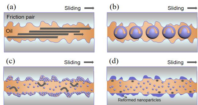
**Fig. 14** Four main friction mechanisms: (a) sliding; (b) rolling; (c) polishing or smoothing; and (d) mending or self-repairing.
