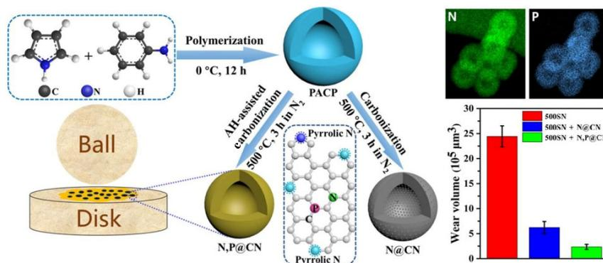
**Fig. 6** Nitrogen and phosphorus co-doped CSs (denoted as CN) were prepared via the carbonization of poly (aniline-co-pyrrole) (PACP), and the prepared CSs with N, P elements showed enhanced anti-wear and friction-reducing performance as 500SN additives. Reproduced with permission from Ref. [83], © American Chemical Society 2020.
