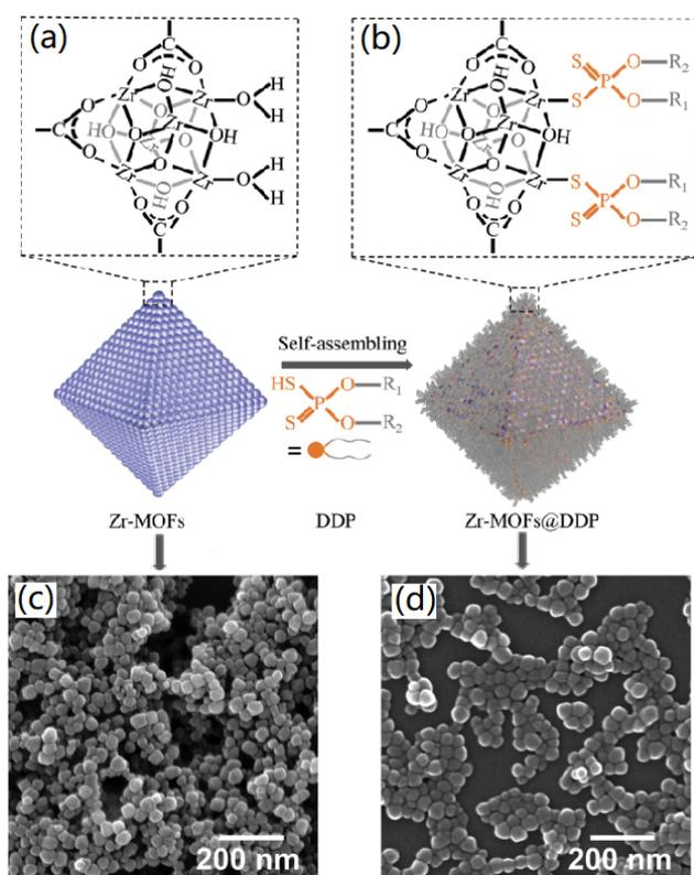
**Fig. 7** Schematic illustration for surface functionalization of Zr-MOFs@DDP. Chemical structures and scanning electron microscopy (SEM) images of Zr-MOFs and Zr-MOFs@DDP were shown in (a, b) and (c, d), respectively. Reproduced with permission from Ref. [113], © Elsevier B.V. 2021.
