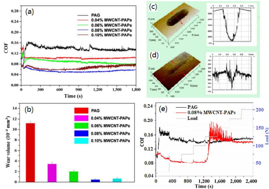
**Fig. 8** (a) COFs and (b) wear volumes lubricated by MWCNT-PAPs with different concentrations (50 N, 25 Hz, and 150 °C); (c, d) three-dimensional (3D) optical microscopic images of the disc worn surfaces lubricated by polyalkylene glycol (PAG) and PAG with 0.08 wt% MWCNT-PAPs, respectively; (e) variations of COF with time under different loads (25 Hz, 150 °C). Reproduced with permission from Ref. [135], © Elsevier Ltd. 2017.
