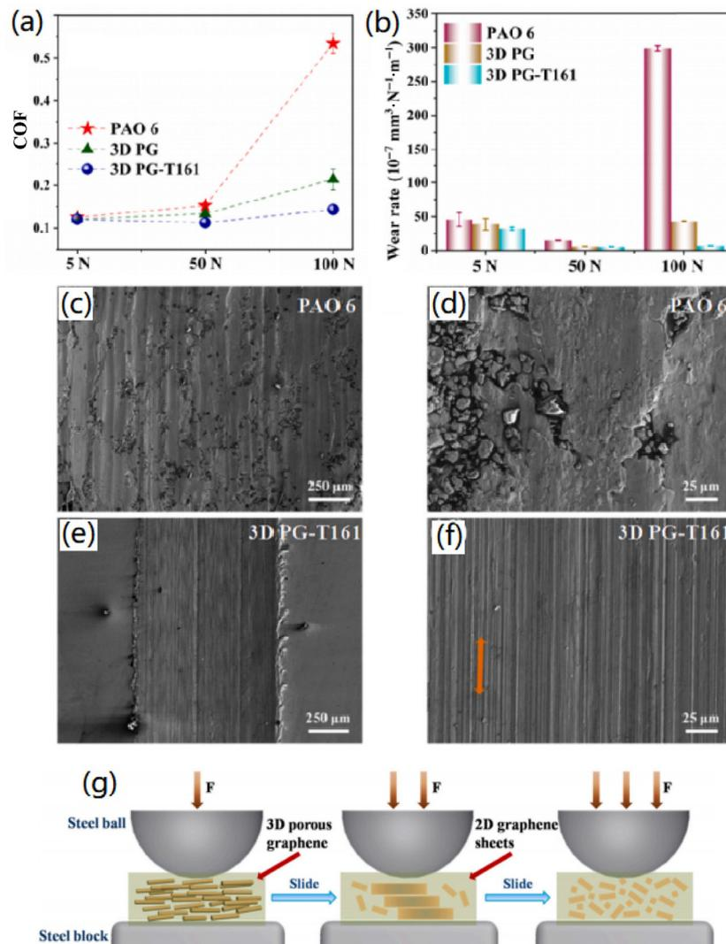
**Fig. 10** (a, b) Changes in average COF and wear rate; (c–f) SEM images of wear track surfaces; and (g) schematic diagram. Reproduced with permission from Ref. [162], © Elsevier Ltd. 2021.
