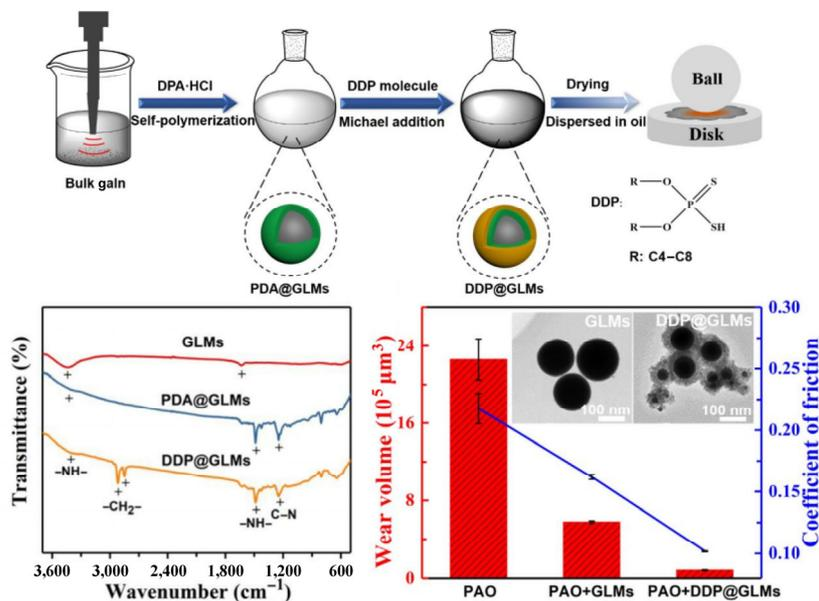
**Fig. 5** Preparation process, FT-IR spectra, and results of tribological tests of DDP@GLMs. Reproduced with permission from Ref. [46], © American Chemical Society 2020.
