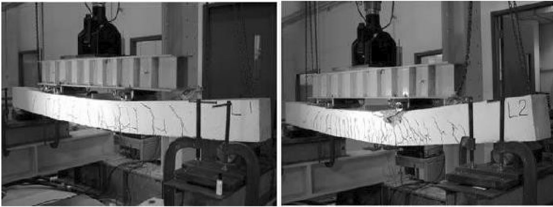
Fig. 9 Cracks patterns for hybrid-reinforced beam [63]
