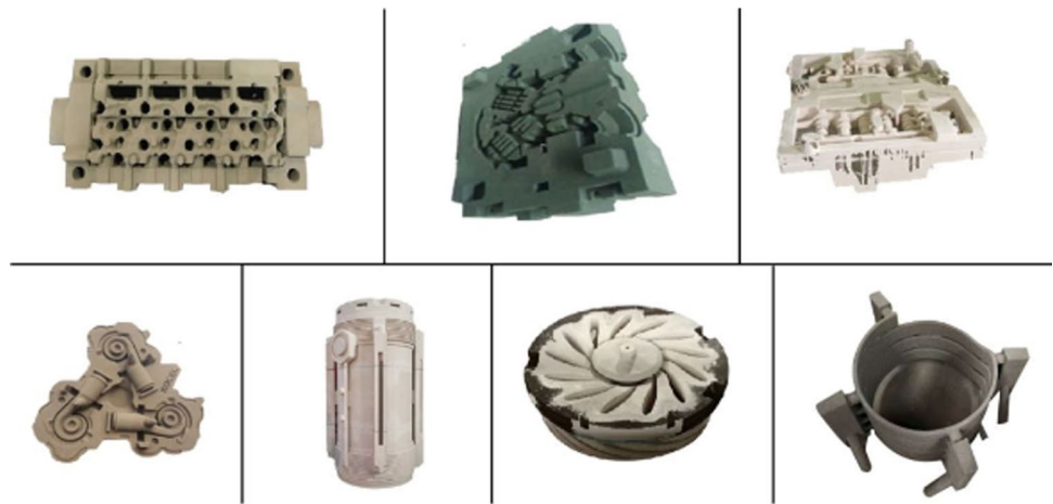
Fig. 3 The application of RSC in developing sand cores and moulds
