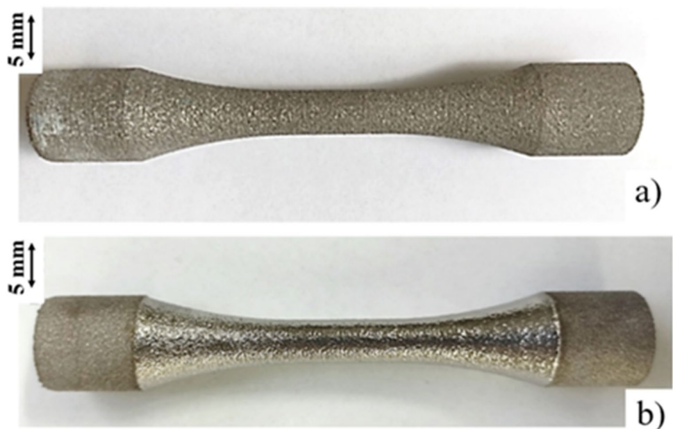
Fig. 10 Pictures of dog-bone samples a before and b after the EP treatment ( \Phi_1 = 35 mm, rpm = 1150, treatment time = 60 min, room temperature, potential = 25 V)
