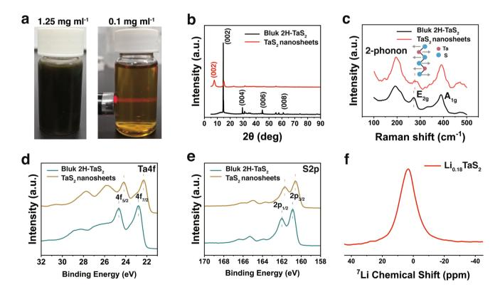
Fig. 2 a Exfoilated 2H- $TaS_2$  nanosheets aqueous dispersions. b XRD spectra of 2H- $TaS_2$  crystals and lyophilized 2H- $TaS_2$  nanosheets. c Raman spectroscopy analysis of the exfoliated nanosheets and the bulk crystal for comparison. XPS high-resolution spectra of d Ta 4f and e S 2p of 2H- $TaS_2$  crystals and lyophilized 2H- $TaS_2$  nanosheets. f  $^7$ Li SP MAS NMR spectra of 2H- $TaS_2$  nanosheets
