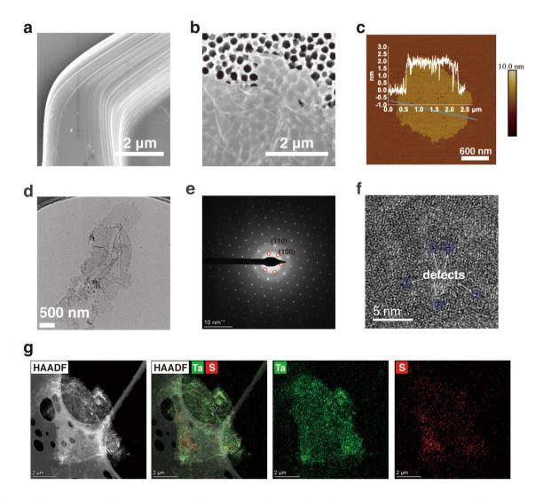
Fig. 3 SEM image of the a 2H-TaS $_2$  crystals and b 2H-TaS $_2$  nanosheets. c A typical AFM image of 2H-TaS $_2$  nanosheets, showing thickness of  $\sim 1.75$  nm. d TEM image, e selected-area electron diffraction (SAED) image, f high-resolution TEM image of 2H-TaS $_2$  nanosheets. g HAADF-STEM and EDS images of 2H-TaS $_2$  nanosheets
