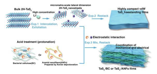
$\textbf{Fig. 1} \ \ \text{Schematic illustrating the preparation processes of } \ \ \text{TaS}_2 \ \ \text{freestanding films, } \ \ \text{TaS}_2 \ \ \text{bacterial cellulose (BC) or aramid nanofibers (ANFs)} \ \ \text{nanocomposite films}$
