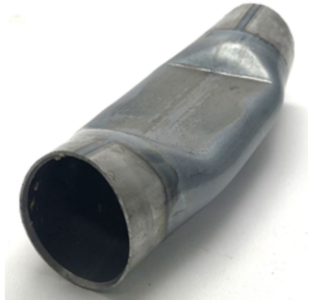
Fig. 17 Hot-stamped tube using a 10 wt% shredded paper fiber-reinforced ice mandrel with three layers of insulation sheets ( n_p=3 ) in flat dies
