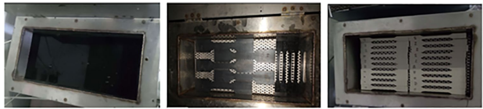
Fig. 3 Direct immersion of specimens in metal bath containing anaerobic digester liquor
