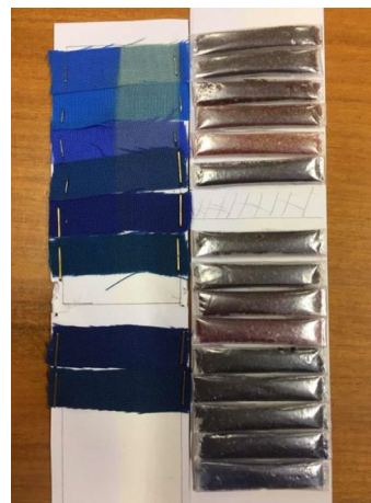
Fig. 11 Imaging of the comparison between dyed retrieved PET particles and the standard “blue”, scale for the study of light fastness
