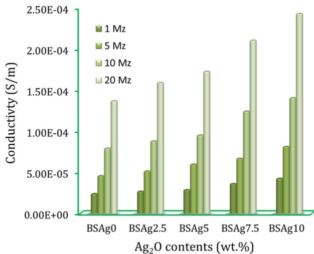
**Fig. 5** AC conductivity of all glass samples with various Ag<sub>2</sub>O concentrations at various frequencies, i.e. 1, 5, 10 and 20 MHz
