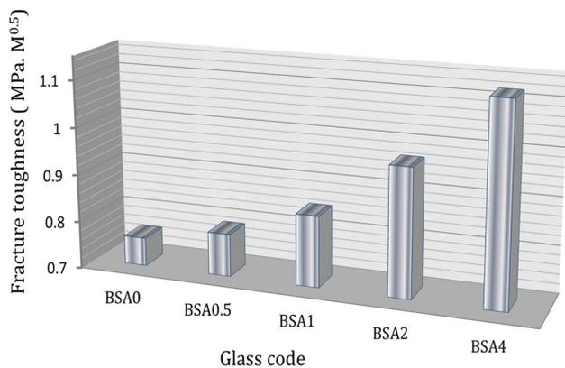
**Fig. 3** BSA0, BSA0.5, BSA1, BSA2, and BSA4 glass samples' fracture toughness
