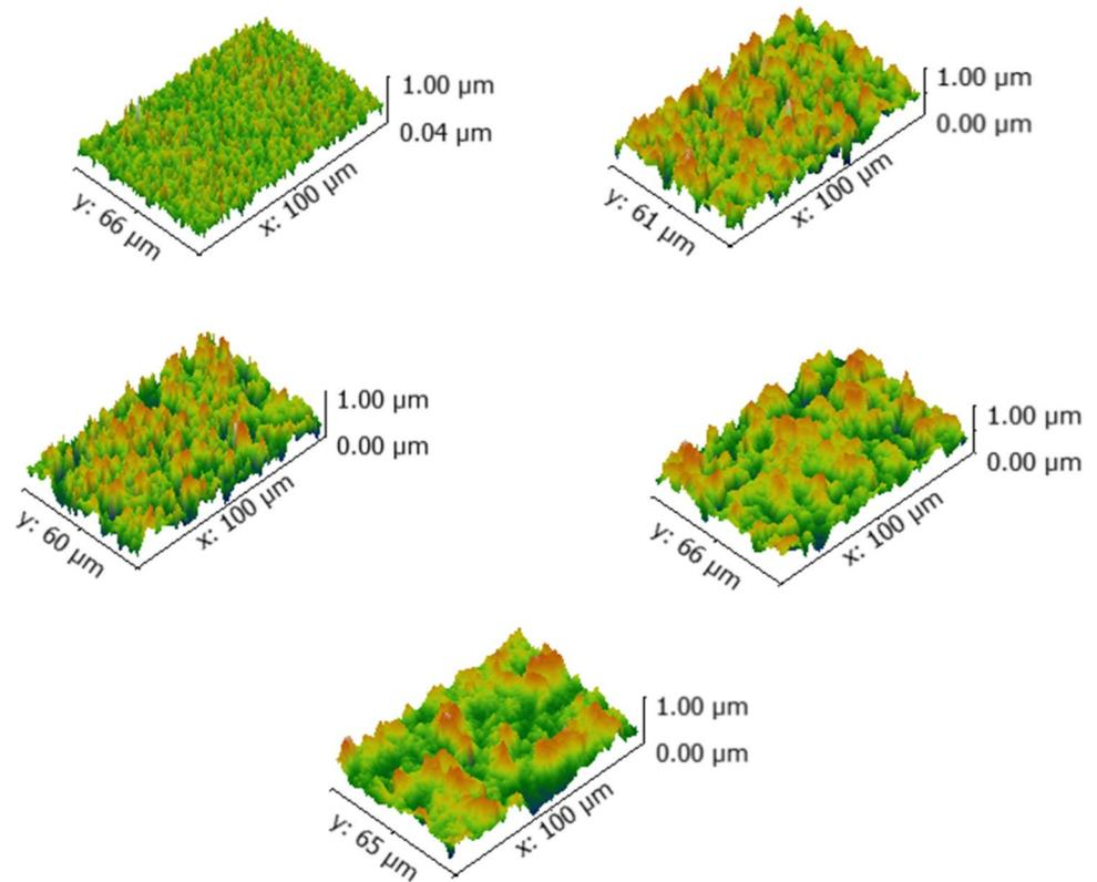
**Table 4** Surface roughness parameters for BSA4 sample before and after soaking in SBF solution for 1, 2, 3, and 4 weeks
