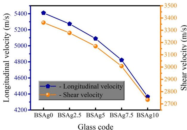
**Fig. 4** Longitudinal and shear velocities of borosilicate glass samples containing Ag<sub>2</sub>O
