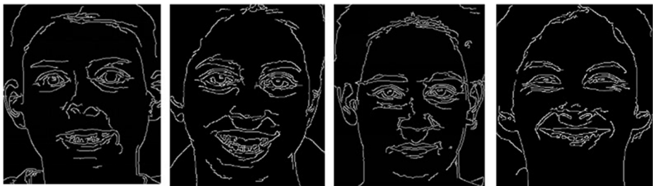
Fig. 3 Edge detection diagram. The network structure constructed in this paper is the input corresponding to the shape of the three-channel image. The input image is processed by the Canny operator to remove noise (The feature map extracted by Canny operator is marked as m ), and combined with the two original pixel feature maps (The two original pixel feature maps are marked as n_1, n_2 respectively) to form a three-channel image ( M = [m, n_1, n_2] ). Then the three-channel image is input into the constructed network for training experiments. This method of combining three-channel feature maps reduces the loss of effective features and improves the recognition accuracy
