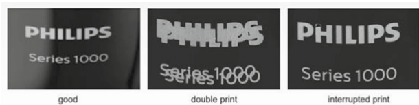
Fig. 6 The images shown above correspond to three possible classes: good (no defect), double print (defective), and interrupted print (defective)
