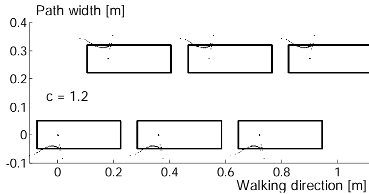
Figure 10. Mechanism footprints of accelerated motion for c = 1.2 . No compensation applied.
