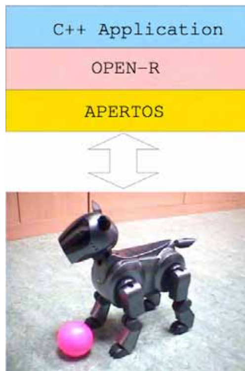
Figure 5. Software architecture for programming Sony Aibo robot
