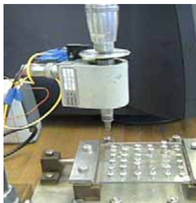
Figure 8. A screwdriver attached transducer and encoder
