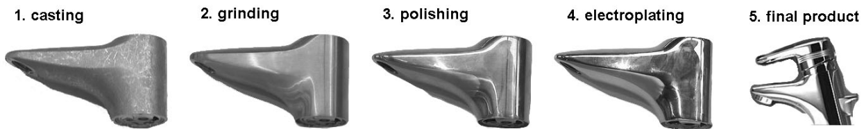
Figure 1. Producing steps in the manufacture of fittings. (1) casting, (2) grinding, (3) polishing, (4) electroplating, (5) end product
