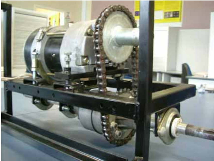
Figure 7. Mounted drive system showing chain tensioning method
