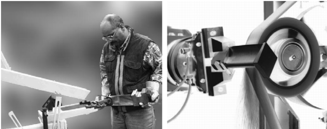
Figure 2. Manual grinding process and robot aided grinding process
