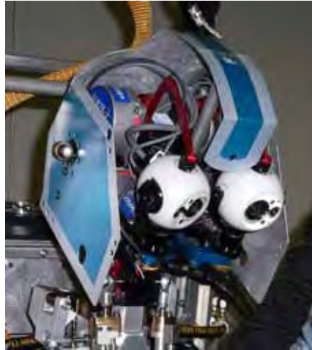
Figure 1. Humanoid head used in the experiments. It has a foveated vision system and 7 degrees of freedom (two DOFs in each eye and three DOFs in the neck)
