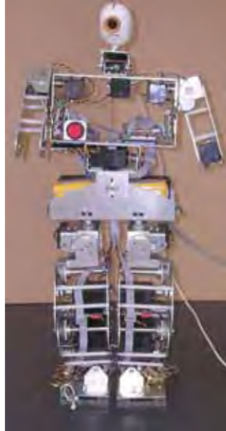
Figure 12. Biped humanoid robot with 22 DOFs
