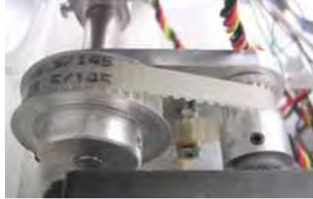
Figure 3. Transmission with a 2.5:1 gear ratio; an adjustable tensile roller holds the belt tight. As mentioned earlier, power to drive the motors is a most relevant issue. Servos absorb high currents, especially at start-up. Two ion-lithium batteries were installed and the system counts with a 7.2 V/9600 mAh pack, with maximal sustained current specified by the vendor at more than 19A. Each one of the two batteries weighs circa 176 g. Proper fusing and charge monitoring were also implemented. Figure 4 shows the selected batteries and their location on the robot.
