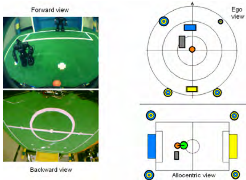
Figure 3. Left: Images of the two cameras mounted on the robot. Upper right: Egocentric coordinates of key objects (ball, goals, corner poles, and obstacle) detected in the image. Lower right: Localization of the robot, the ball, and the obstacle on the soccer field
