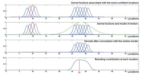
Figure 8. Improvement of the localization phase through a probabilistic-based approach. The new location depends on the previous one and the image acquired
