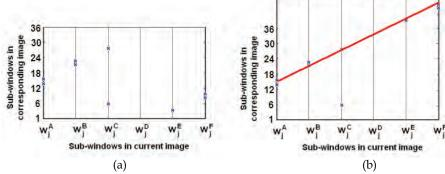
Figure 10. Computing the steering speed of the robot with the sub-windows approach. This speed is proportional to the ordinate in the origin of the fitted line
