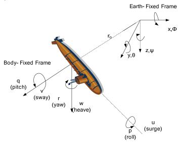
Figure 2. Earth-fixed frame and body-fixed frame for AUV
