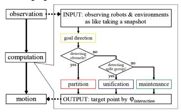
Figure 10. Adaptive tracking flowchart
