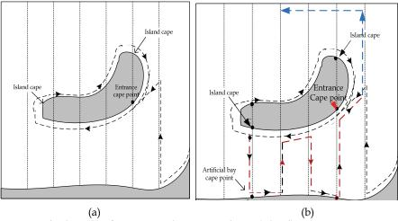
Figure 10. Hert's algorithm for non-simply connected area (island)
