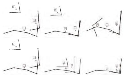
Figure 7. The top row shows 3 steps of the alignment of 3 scans (each scan consists of a single corner only) by classical ICP, the bottom-row shows the results of the proposed approach. The alignment progress can be seen from left to right in both cases. The square boxes show the robot poses of the the scans
