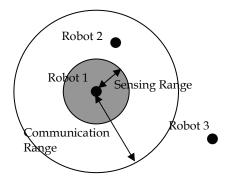
Figure 2. Schematic diagram showing the sensing and communication ranges of a robot For the target search problem, there are two major tasks: (1) the dispatch manner at the base station, and (2) the dispersion manner on each individual robot.
