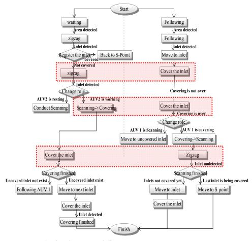
Figure 16. Simulated Multi-AUV work flow
