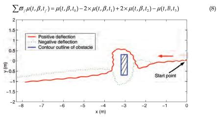
Figure 8. Simulated trajectory for a simple obstacle-avoidance case
