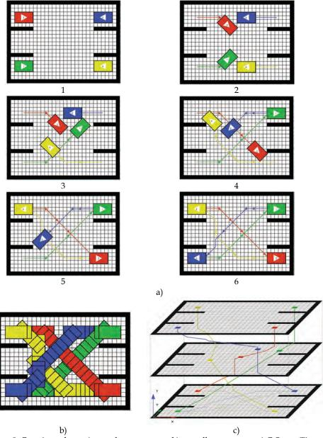
b) c) Figure 9. Crossing robots: a) snapshots sequence; b) overall movements; c) C-Space-Time movements (planning time: 1.26 s, 897′600 cells)
