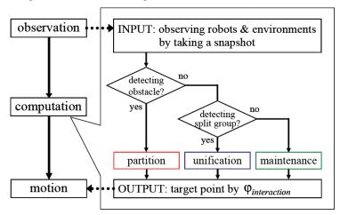
Figure 3. Adaptive flocking flowchart
