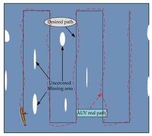
Figure 1. AUV missing areas caused by complex disturbances
