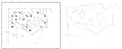
Figure 10. Left, final map (after 50 iterations) of intialization fig. 9 with FFS. Right, the final map obtained by the Lu & Milios technique as reported in (Borrmann et al., 2007). The systems lead to results of comparable quality
