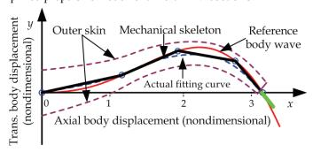
Figure 2. Actual fitting curve versus reference body wave in the multi-link robotic fish model Fish is composed of tens of vertebra, as is observed, and each vertebra may be regarded as a miniature joint. The oscillatory part of the robotic fish, in this sense, could be discretely designed as a multi-link (or *N*-link) mechanism which consists of several oscillating hinge
