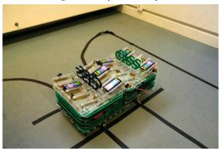
Figure 9. Two robots in a battery exchange process
