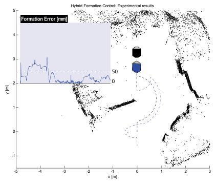
Figure 14. Experimental results: formation control with obstacles
