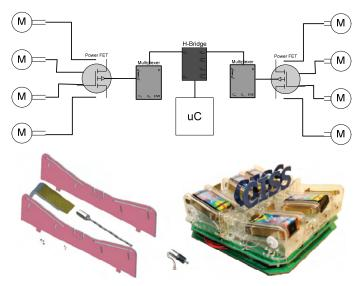
Figure 20. Battery pushing system: block diagram (Top), diassembled mechanical part (bottom left), geared micro-motor (bottom middle), completed system (bottom right)
