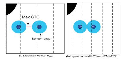
Figure 12. Calculating of EEW using CTE
