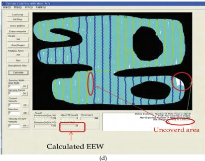
Figure 20. Multi-AUV simulated the covering method in an unknown terrain without EEW by following steps: (a) The AUV starts covering to detect cape. (b) Two AUVs define coverage roles.(c) Two AUVs change role considering coverage situation.(d) Results after completed coverage
