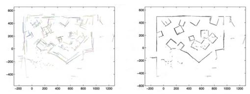
Figure 2. Left: Pre-alignment of the 60 scans of the NIST disaster test area. Right: improved alignment. Force Field Simulation is used to achieve the improved alignment, given an estimated pre-alignment
