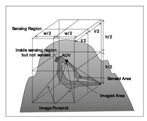
Figure 4. Illustrated AUV sensing model in underwater environment
