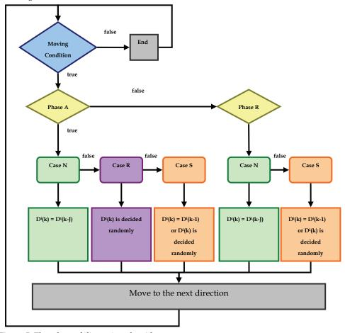
Figure 5. Flowchart of dispersion algorithm
