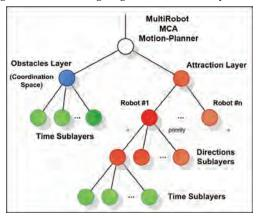
Figure 3. MultiLayered Motion-Planner Architecture
