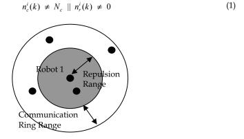
Figure 4. Schematic diagram showing the repulsion and communication ranges of a robot
