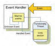
Figure 2. The core of a module: the event-handler
