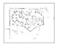
Figure 9. left: 60 scans superimposed building a global map using a rough initial transformation estimation, right: after 20 iterations of FFS. The crosses show the robots' positions, (the reader might try to find the 6 single scans of fig. 8 in the global map. 1,2,3 and 6 are part of the upper left corner, 4 and 5 are located in the lower left corner). The final result of FFS is shown in fig. 10, left
