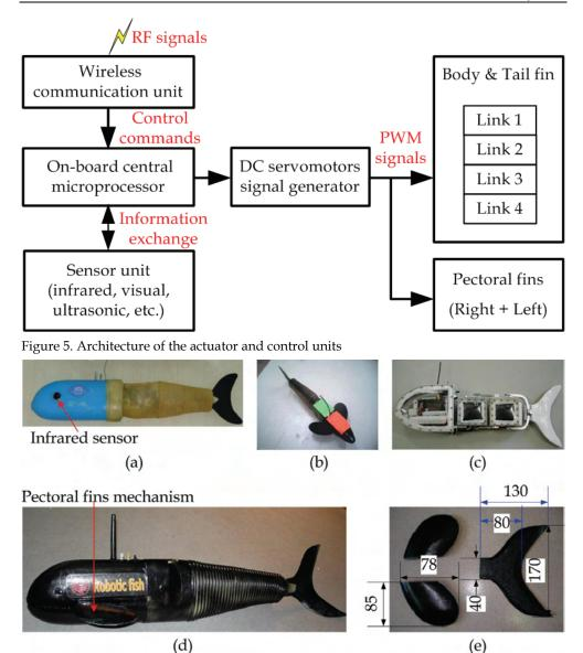
Figure 6. Prototypes of different robotic fish. (a) Four-link robotic fish equipped with infrared sensors, 405 mm in length; (b) three-link robotic fish, 380 mm in length; (c) two-module, reconfigurable robotic fish; (d) four-link, multimode robotic fish with the capability of autonomous three-dimensional (3-D) swimming, 650 mm in length; (e) shape and dimension of both pectoral and caudal fins of the multimode fish
