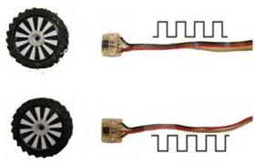
Figure 16. Odometer: barcode (left), short-range infrared sensors (right)
