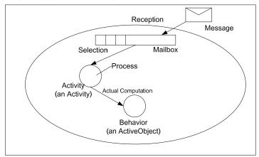
Figure 1. Components of an Actalk active object
