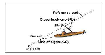
Figure 11. Illustrated cross track error by AUV
