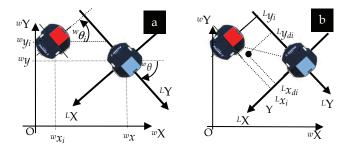
Figure 1. a) Reference systems: world (absolute) reference coordinate system (O  ${}^w$ X  ${}^w$ Y), and a second coordinate system attached to the leader robot (O  ${}^L$ X  ${}^L$ Y) where the desired positions for each of the followers are defined. b) i-th follower robot positioned at coordinates ( ${}^L$ x<sub>i</sub>,  ${}^L$ y<sub>i</sub>) on the leader Cartesian reference where the reference position is given by ( ${}^L$ x<sub>di</sub>,  ${}^L$ y<sub>di</sub>)
