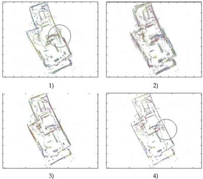
Figure 11. Apartment data set. 1) initial configuration. The circled area shows an error due to incorrect loop closing. 2) A large step parameter dT blurs the map in the first iteration step to escape from the local minimum 3) iteration 50: 4) iteration 150: FFS has not only contracted the edges given in 1), but also has realigned the entire global map to fix the error (circled area)
