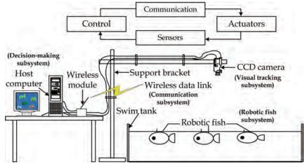
Figure 15. Hardware platform for the MRFS
