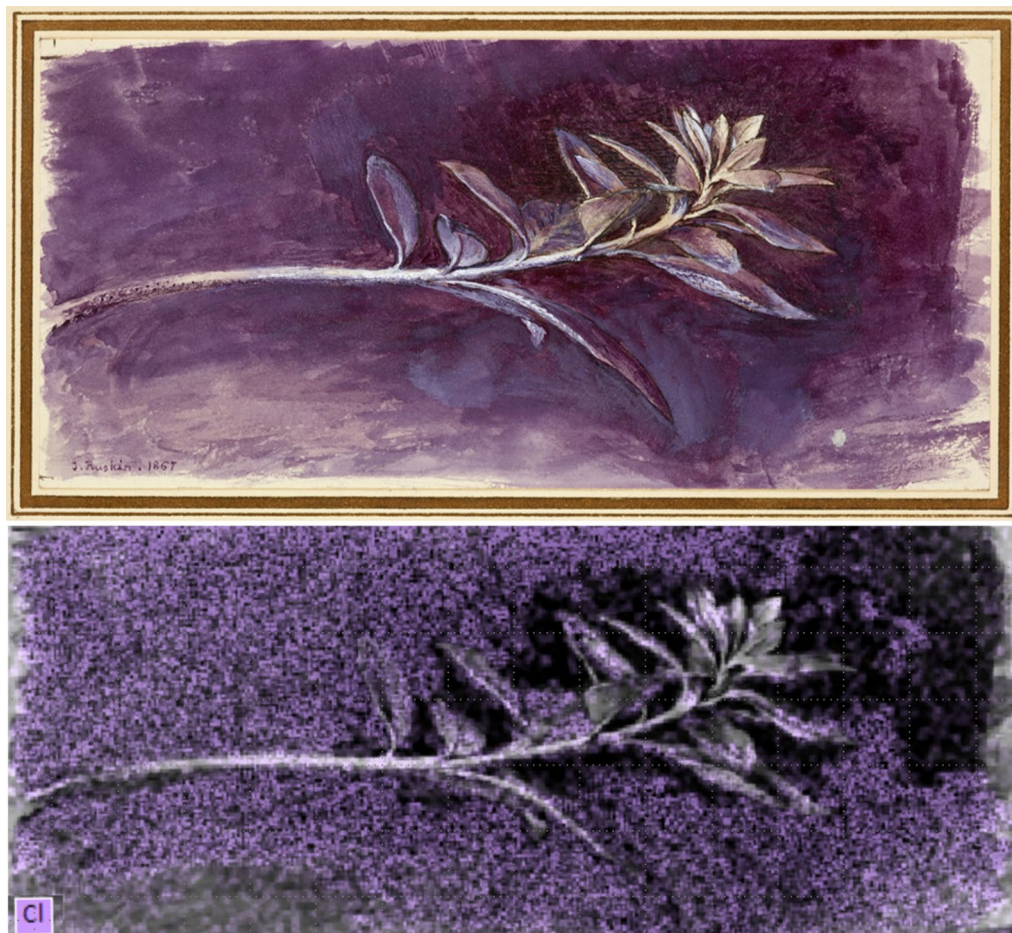
Fig. 10 Top: Growing Shoot of Mock Privet (WA.RS.ED.267). Bottom: macro-XRF maps of chlorine overlapping a stitched image of the watercolour
