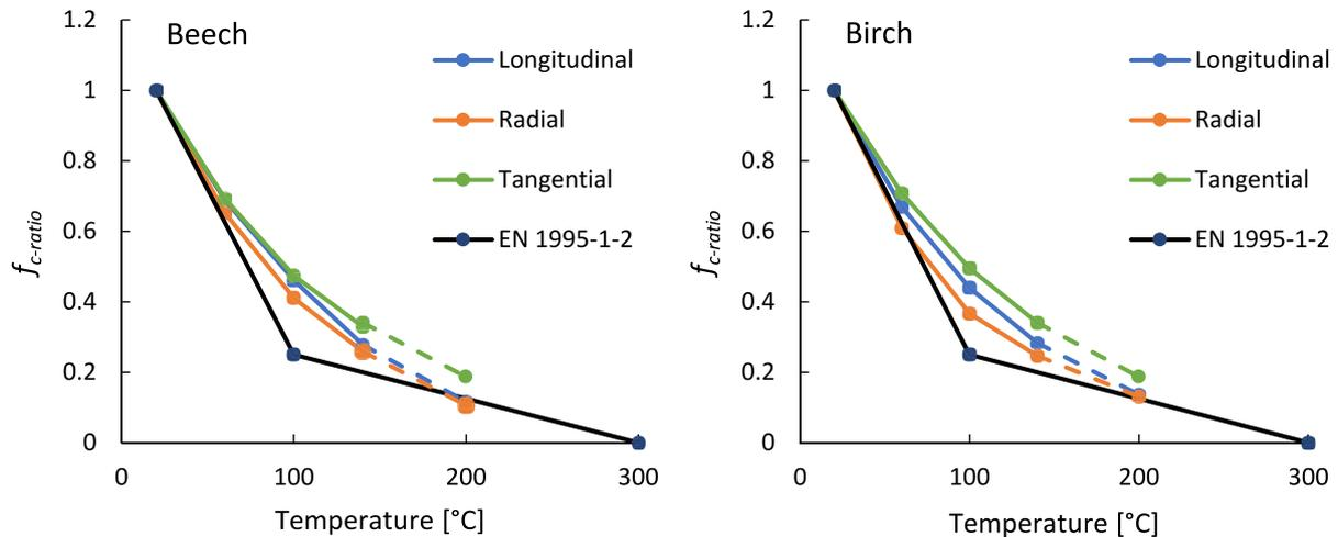
**Figure 10** Comparison between  $f_{c-ratio}$  presented in the Eurocode and estimated  $f_{c-ratio}$  of beech and birch with temperature.
