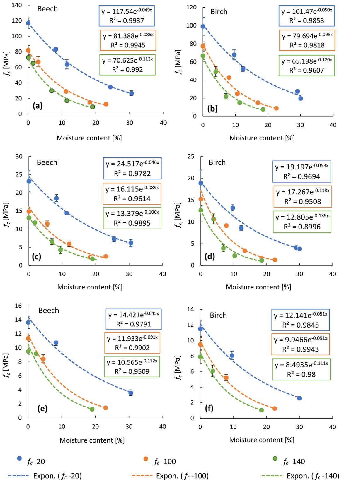
**Figure 2** Compressive strength ( $f_c$ ) of beech and birch with moisture content at different temperatures (20, 100 and 140 °C) in: **a**, **b** longitudinal; **c**, **d** radial and **e**, **f** tangential directions.
