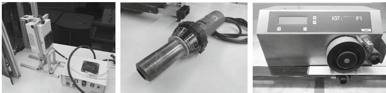
Fig. 2: Set-up for UV-curing (left), hot air blower (middle), and laboratory flexo printing machine IGT F1 (right) used in the experiment
