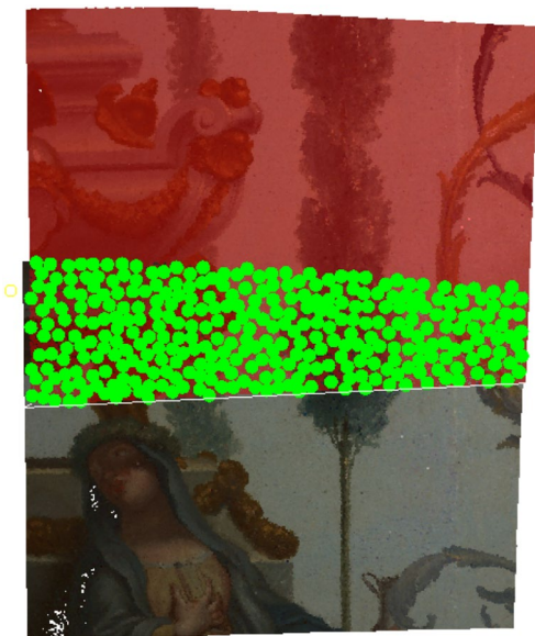
Fig. 23 Control points marked on the overlapping region between stable and transformed point clouds
