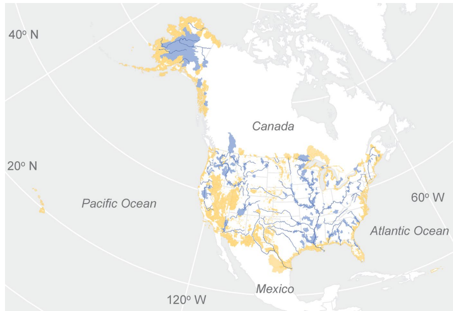
Fig. 3 Incremental gaged areas in the USA and bordering areas where the absolute value of incremental median annual minimum daily streamflow > 12.7 m 3 /s (blue areas) indicating low network resolution, 12-digit hydrologic unit code watersheds where more than 50% of their area is unmonitored (orange areas) indicating gaps in network coverage, and major rivers with drainage areas > 10,000 km 2 (blue lines)
