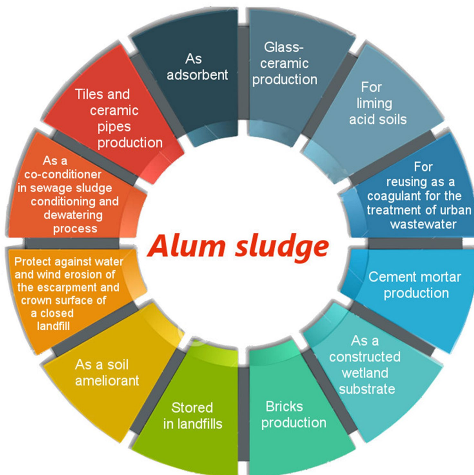
Fig. 2 Various directions of use and management of AS (Ahmad et al. 2016; Babatunde and Zhao 2007; Babatunde et al. 2008; Balkaya 2015; Dassanayake et al. 2015; Guan et al. 2005; Kim et al. 2002; Lombi et al. 2010; Nair and Mansoor Ahammed 2015; Tarrago et al. 2017; Yang et al. 2006a; Zhao et al. 2009, 2011)
