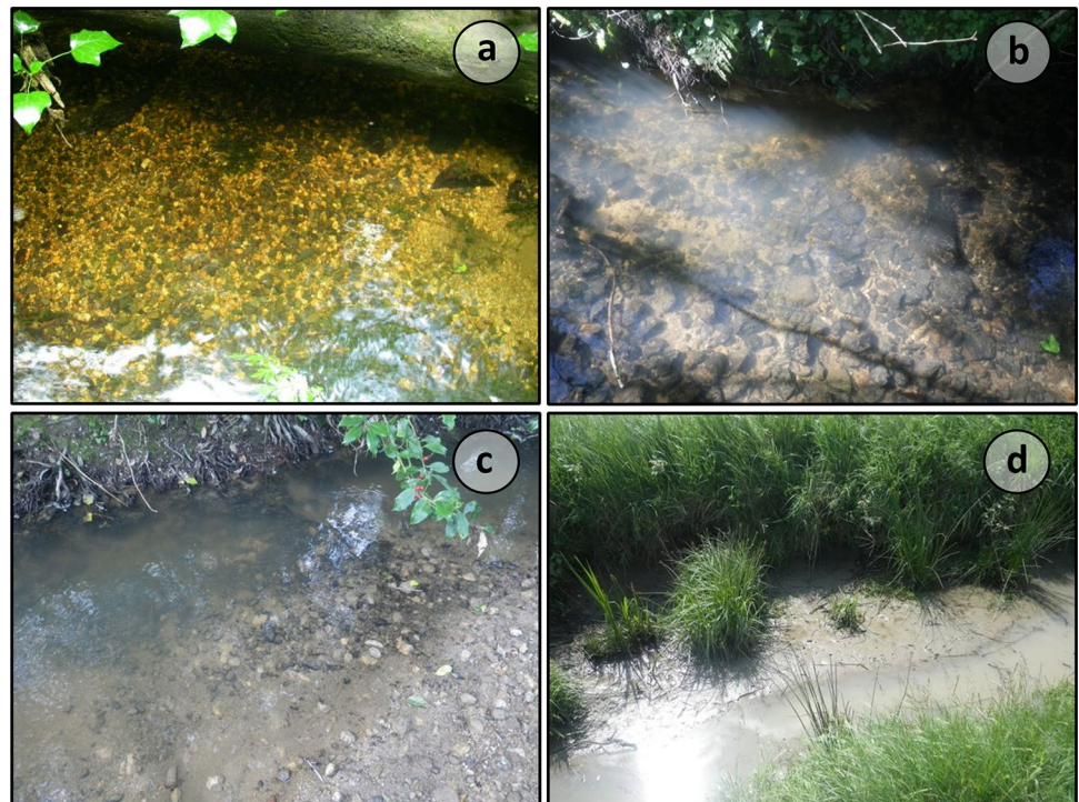
Fig. 2 Illustrations of different sediment deposition intensity classes, in increasing order, as estimated in the field. a No fine sediment (0%), b weak intensity (25–50%), c moderate intensity (50–75%), and d high intensity (75–100%)
