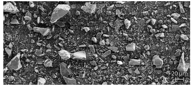
Fig. 15 SEM image of glaze powder after sieving
