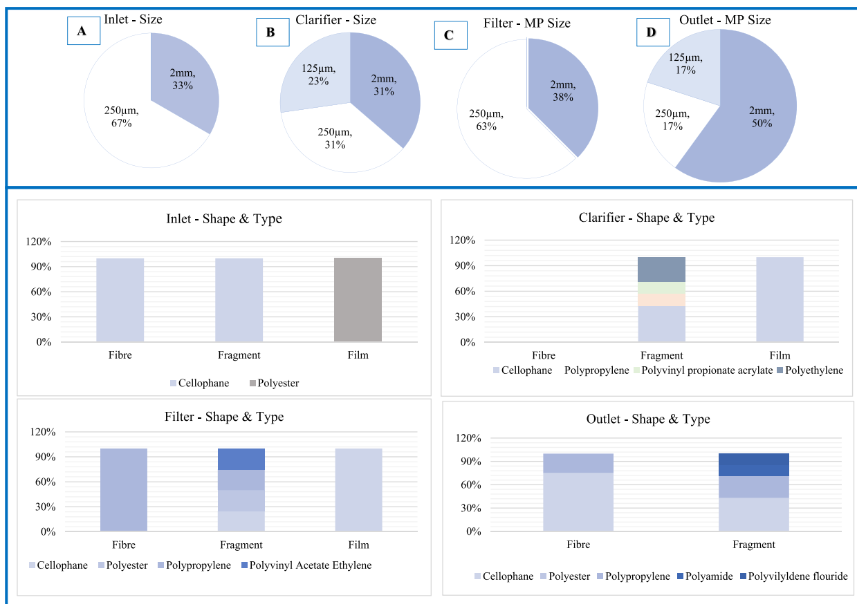
Fig. 3 The pie chart shows the different percentage of sizes of MP’s captured from the different stages of treatment in Kinoya WWTP and the percentages of different types of shapes captured in the bar graphs
